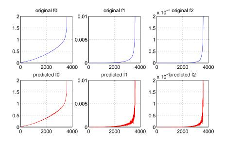
Figure 7-5: Approximated data (local third-order polynomials) from a simulated amplifier:  $b_2(1), b_2(2), b_2(3)$ . The x-axis gives the test event, the y-axis indicates the energy in the component. Original and predicted output data are sorted individually by the energy of the particular component. The noise (non-monotonicity) in the predicted  $f_1$  and  $f_2$  plot indicates a slight prediction error.
