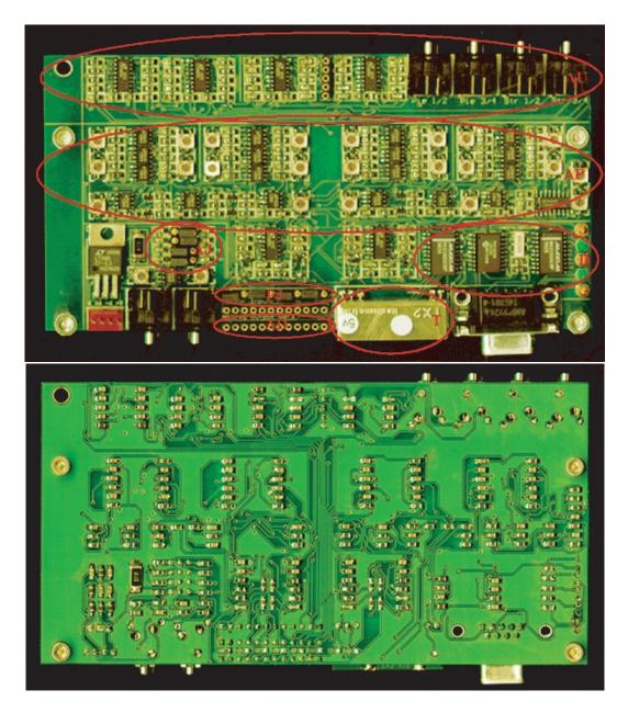
Figure B-3: Violin/cello sensor board. Front and (vertically flipped) back. **AP**: analog processing; **AU**: audio processing; **D**: digital processing; **T**: transmitter unit; **AD**: connector for analog data; **PJ**: power off jumpers; **AJ**: antenna jumpers.
