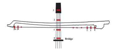
Figure B-5: Grid of measurement points in x and y direction for the bow calibration.
