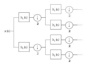
Figure 4-4: Wavelet packet transform. Implementation of the filter bank:  $h_0(n)$  and  $h_1(n)$  are the half band low-pass and high-pass filters,  $2 \downarrow$  stands for down-sampling by a factor 2.
