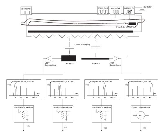
Figure B-6: Functional diagram of the bow sensing technology.
