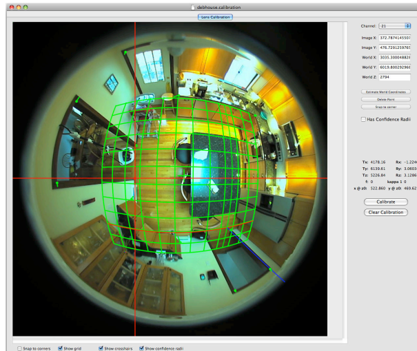
Figure 17. The interface used for camera calibration. Rony Kubat developed the interface, and I developed the camera model and parameter solver.
