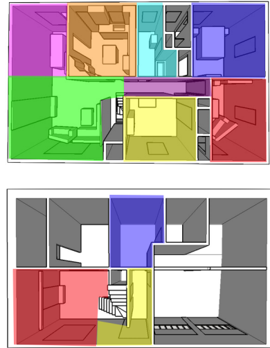
Figure 16. Partitioning of the environment geometry into zones, each of which is textured by a single camera.
