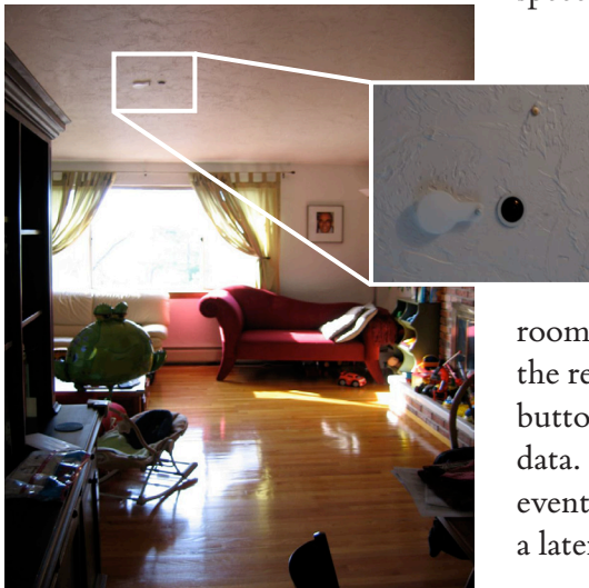
Figure 6. A camera and microphone mounted in ceiling. The microphone is the small silver button near the top.
