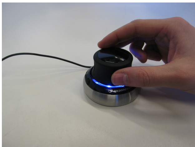
Figure 5.3: The 6-DOF input device used to enter the six head pose parameters.
