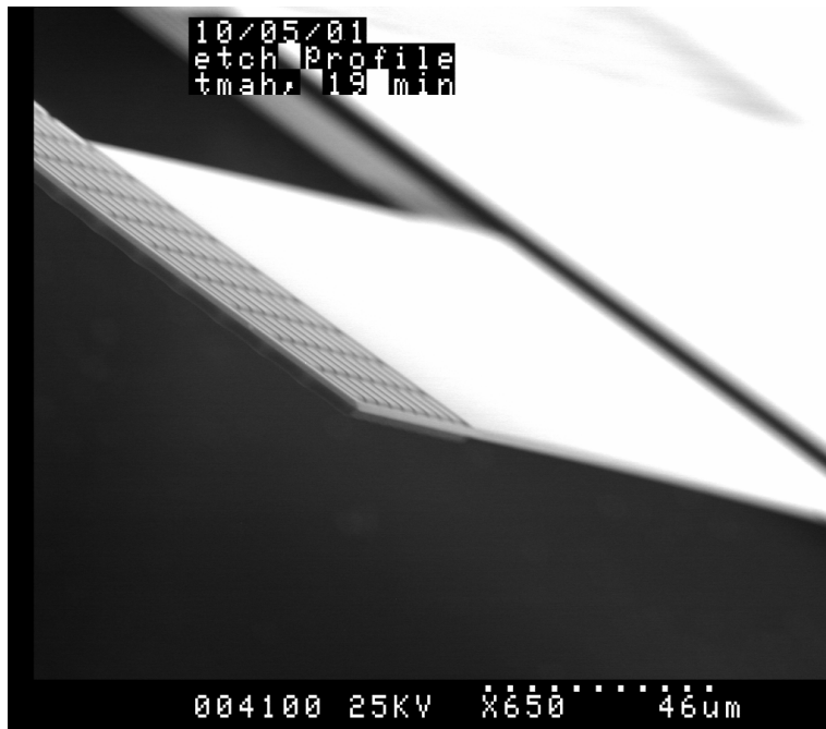
Figure 4.2.11. SEM view of the (honeycomb support)-(sensor cantilever) junction
