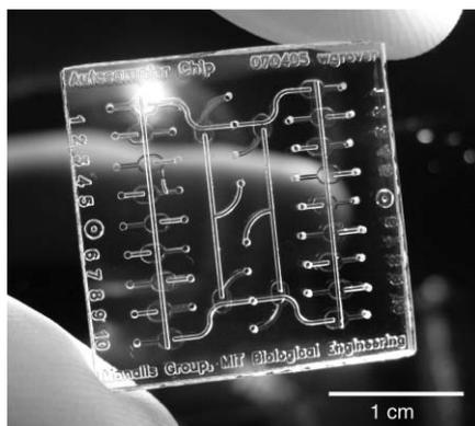
**Fig. 1** Photograph of an Autosampler Chip containing 22 FEP Teflon monolithic membrane valves. The Autosampler Chip can deliver extremely caustic piranha solution (concentrated sulfuric acid and hydrogen peroxide) to clean an off-chip sensor without causing any detectable damage to the chip or its valves.<sup>23</sup>
