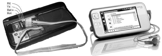
Figure 2: The Nokia N800 (right), with serial port exposed in an open back to show our custom adapter (left)
