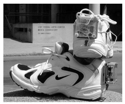
Figure 5. Piezoelectric-powered RFID shoes with mounted electronics.
