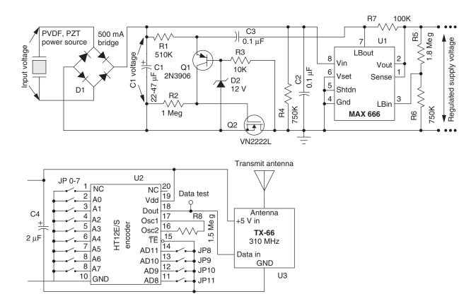
Figure 6. Schematic of power-conditioning electronics and encoder circuitry for the shoe-powered RF tag system.
