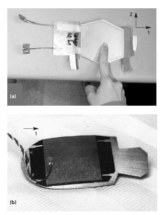
Figure 3. View looking down at the PVDF insole stave (a) and the PZT dimorph heel insert (b). In both views, the right side of the device is pointing to the shoe's toe.
