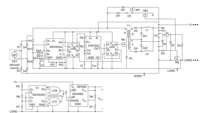
Figure 8. Forward-switching converter system.
