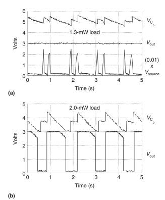
Figure 9. Switching converter signals for a continuous 1.3-mW load (a) and a 2.0-mW load (b), showing low-voltage shutdown. Both examples resulted from walking with the PZT dimorph source, represented in the bottom plot of (a).
