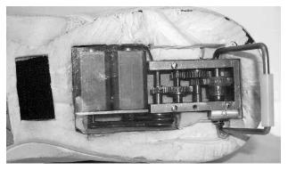
Figure 10. Pair of rotary magnetic generators embedded in a sneaker sole with step-up gear mechanisms.
