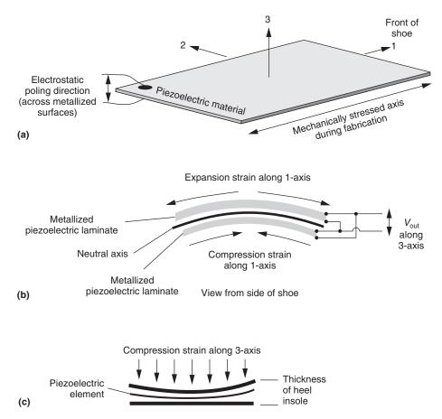
Figure 1. Conventional axis definition for a piezoelectric material (a). Our applications rely on 31mode (b) in bending. The 33-mode (c)—when the heel motion in the 3-axis direction compresses the shoe's sole and induces an electric field along the same axis—is intuitively appealing but inefficient because of the small integrated strain across the thickness dimension (3-axis).
