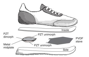
Figure 2. Two approaches to unobtrusive 31-mode piezoelectric energy scavenging in shoes: a PVDF stave under the ball of the foot and a PZT dimorph under the heel.
