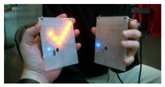
Figure 6. The badge at right has bookmarked the badge at left - blue LEDs signify an encounter in progress and the checkmark verifies the bookmark. Note that this early version of the badge lacked the easier-to-use front-mounted buttons and only used the side-mounted switch.
