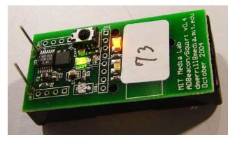
Figure 4. The "Squirt" - a compact IR tagging beacon
