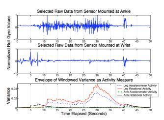
Figure 5. Selected data and resulting activity envelopes as dancer transitions from slow kicks to rapid tense kicks. Sequence of leg motions is framed by stylistic arm motion.
