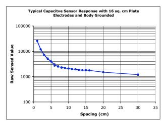
Figure 8. Typical response of the capacitive sensing system.
