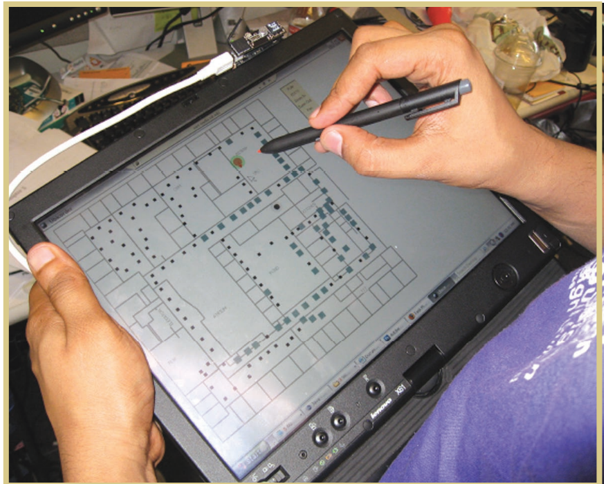
Figure 9. The Ubicorder. The electronics package at the tablet's upper right contains the compass and accelerometers used for pointing, together with the 802.15.4 radio and IR link for communicating with the portal sensor nodes.
