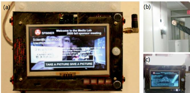
Fig. 6. (a) Cloud of Images application. (b)(c) After pressing the “TAKE A PICTURE GIVE A PICTURE” button, bright onboard LEDs light up for illumination.
