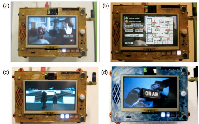
Fig. 4. (a) Awareness App in idle mode - the screen plays canned video content, such as movies appropriate with the theme of a hosted event (b) when activated, the application presented a map of the building on the portal’s touch screen (c) Rendering of the UMPs corresponding virtual location in Second Life. (d) The remote UMP displays an “on-air” indication notifying nearby individuals that video is being streamed to another location in the building.
