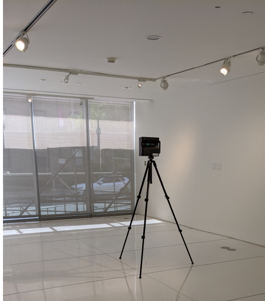
Figure 5-6: For scanning the environment, we first setup the matterport in a tripod and place it in the space we want to scan.
