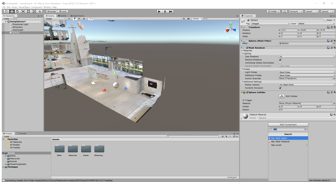
Figure A-12: Add the Unity NavMesh Agent component into the Sphere or the embodied character.
