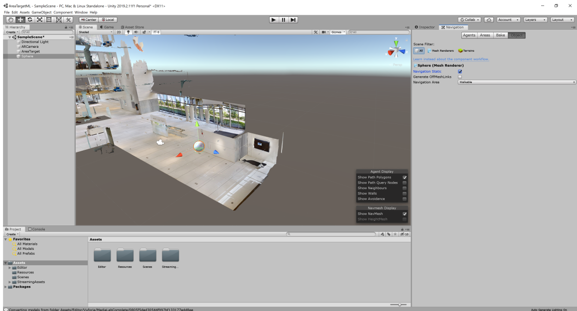
Figure A-15: Enable Navigation Static under the navigation tab next to the Inspector Tab.
