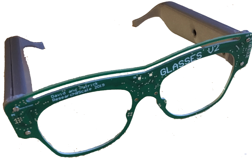
Figure 3-1: Initial Design of Glasses with Three Rigid PCBs
