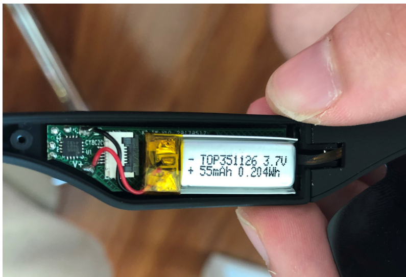
Figure 3-7: Battery on One Side of Glasses
