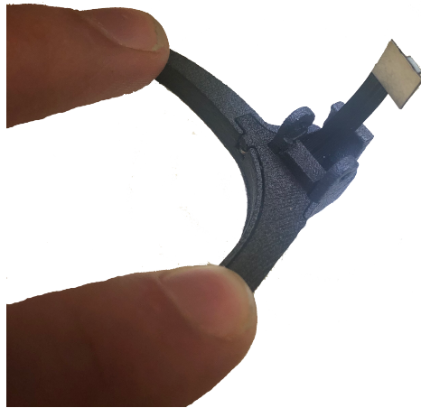
Figure 3-21: Sealed Front Housing with Flex Circuit Integrated
