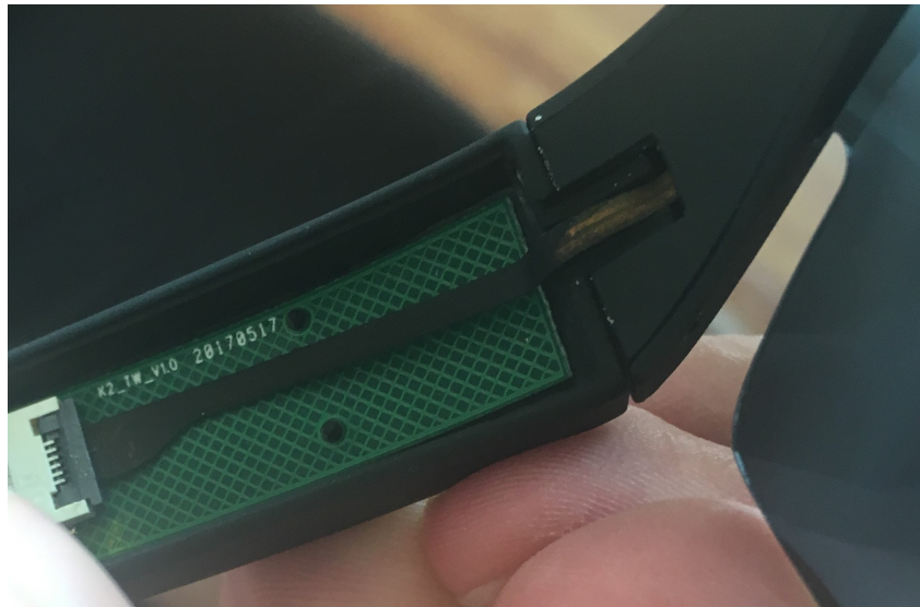
Figure 3-4: Flexible Circuitry Running Through Hinge of a Common Smart Eyeglass Architecture
