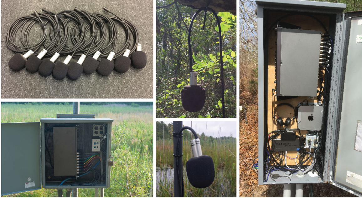
Figure 2-4: Parts of the audio streaming installation. Top left: microphones awaiting installation. Bottom left: satellite input box. Center: microphones in trees and in the marsh. Right: main electrical box, showing mixer (top), computer (center), network switch and fiber (bottom left). Figure excerpted from [86].
