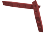
Figure 4-70. Model of two tiles in a metastable bond, requiring a swivel bearing mechanism or low-friction surface (e.g., Teflon) to re-align.
