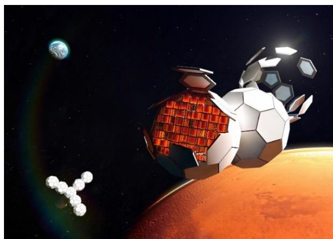
Figure 6-37. Artist’s render of TESSERAE logistic and storage concept, at scale, in orbit around Mars for a prospective MOSAIC (Mars Orbiting Self-Assembling Interlocking Chambers) mission. Image courtesy of TU Dortmund Fraunhofer Institute, for TESSERAE.
