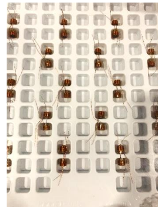
Figure 4-47. Left: Force vs Air Gap curve for the chosen design, showing attraction (orange) and repulsion (blue). Right: EPM units delivered in 75 N-S exposed pairs, for 150 total units.
