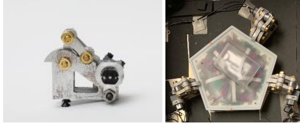
Figure 4-27. Left: Close-up of suborbital launch latch mechanism. Right: Three latches in action, securing pentagon TESSERAE tile for flight. Designed by Peter Dilworth.
