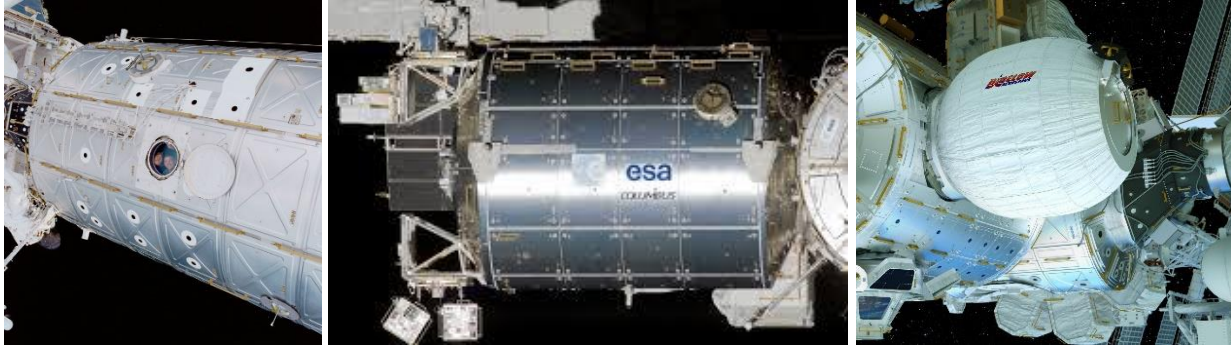
Figure 6-20. Comparison photos of the cylinder-dominated Destiny (left), Columbus module (center), and the ellipsoid inflatable BEAM (right). ISS module specifications are drawn from Columbus, 213 Destiny, 214 BEAM. 215
