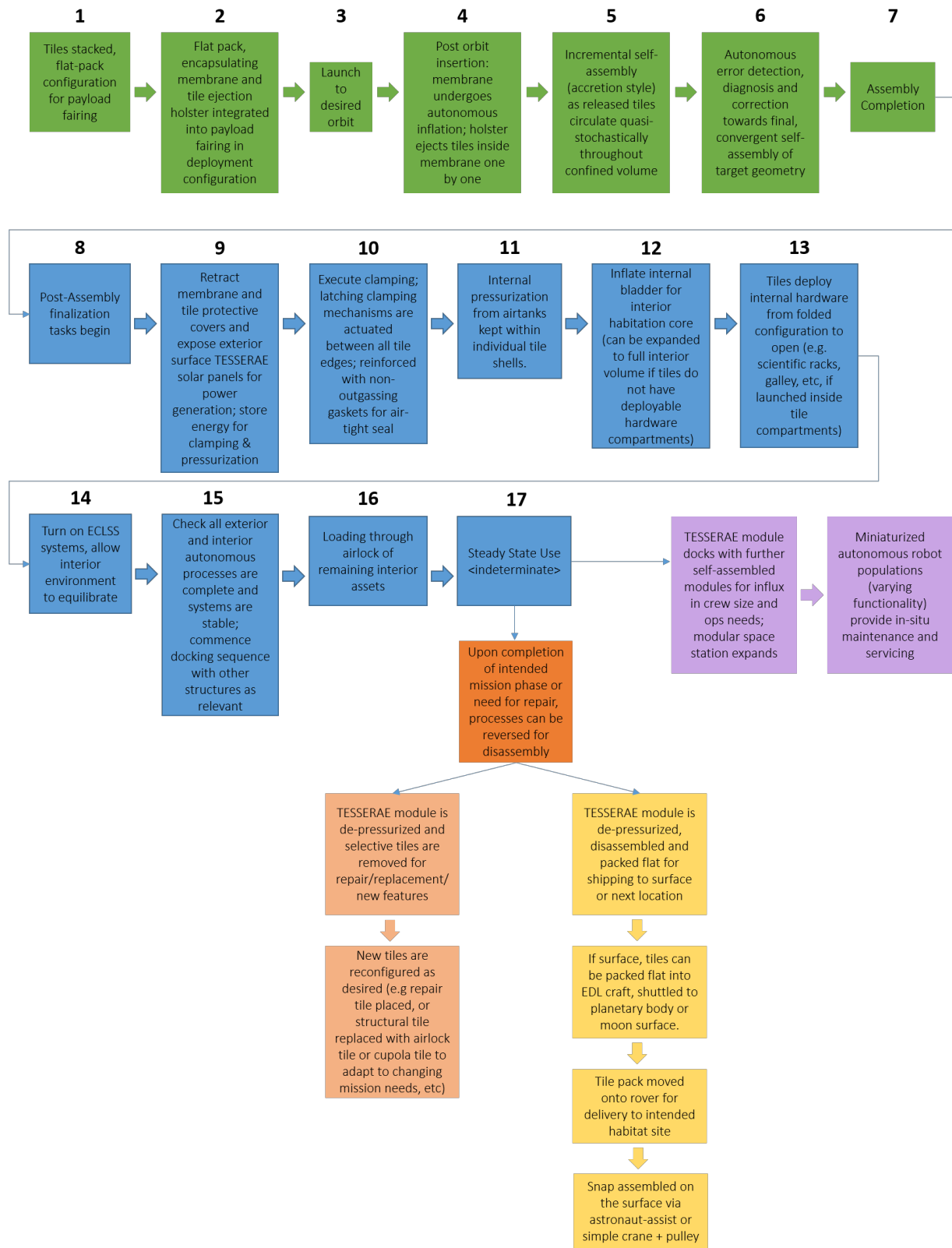
Figure 6-6. Flow chart tracking step-by-step deployment for TESSERAE self-assembling habitat system, including pre-launch to assembly (green, 1-7), post-assembly finalization tasks (blue, 8-17), and end-use cases in orbit or on a planetary/moon surface. See arielekblaw.com/tesseract for an illustrative video depicting this deployment and hybrid use.
