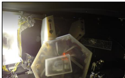
Figure 4-33. Two Gen 2 tiles inside the Blue Origin chamber bonded without completely obscuring the proximity slot; ISS hardware and control code was updated to correct for this and rely instead on the magnetometer for bonding event detection and first-pass diagnosis.
