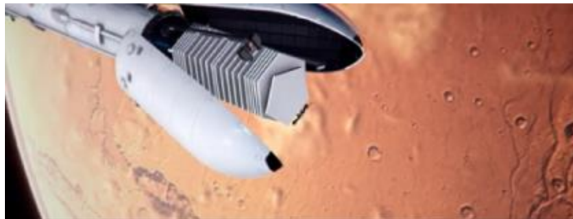
Figure 6-9. Speculative view of TESSERAE tiles packed flat in deployment holster in Spiral Arm insertion order, ready for payload fairing separation in orbit around Mars. Image Credit: TU Dortmund Fraunhofer Institute, for TESSERAE.
