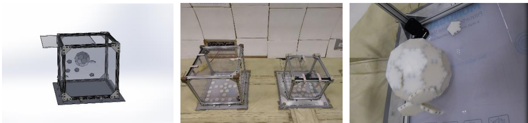
Figure 4-15. Experimental test apparatus for microgravity flight (Left/Center), assembly behavior during flight (Right).
