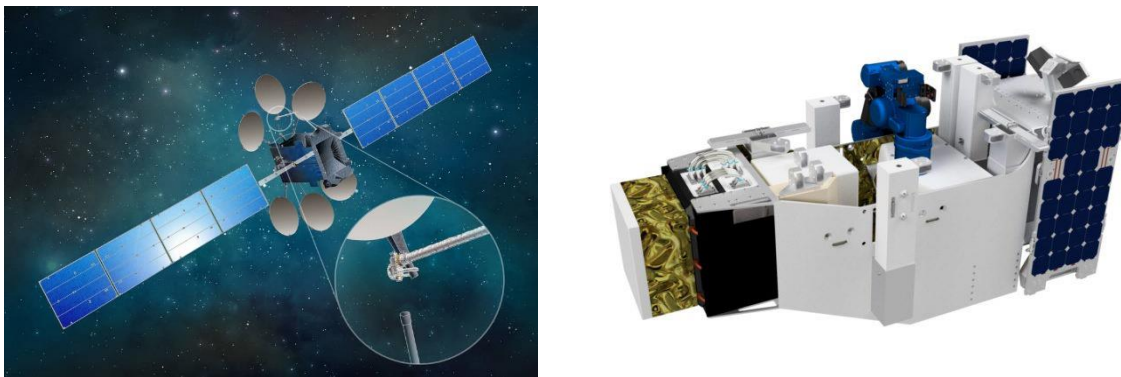
Figure 6-39. Related robotic, on-orbit assembly plans with which the TESSERAE Platform could partner. Left—NASA’s 2017 conception of a modular, self-assembling satellite. 251 Right—Made in Space’s Archinaut system for additive manufacturing and robotic assembly on-orbit (image credit: MIS). 252
