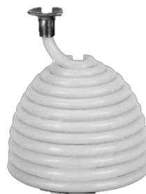
Figure 6-41. Sample extrusion model process with bonded coils.
