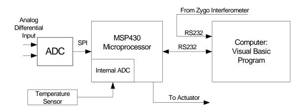
**Figure 17: Data Acquisition System**
