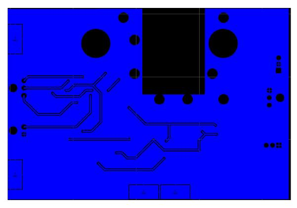
Figure 41: Analog front-end PCB layout, bottom layer
