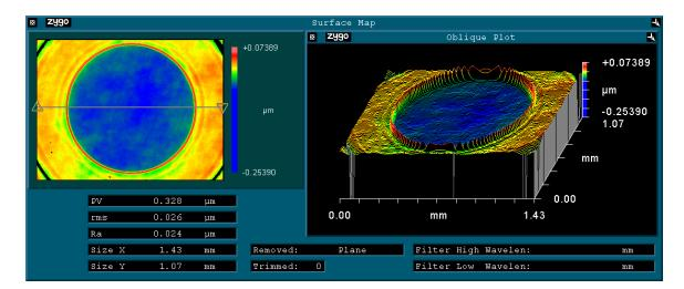
Figure 10: Profilometer scan of the Pyrex wafer after bonding. The reflow of the Pyrex wafer can be seen conforming to the shape of the silicon valveland. The remains of the fulcrum can be seen at the corners.
