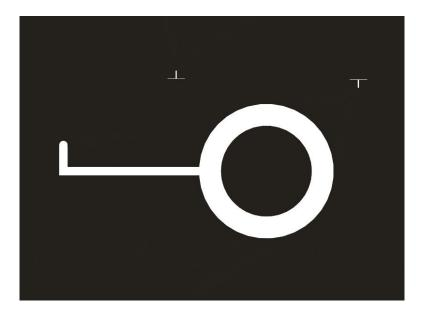
Figure 5: Capacitive electrode mask for the Pyrex wafer
