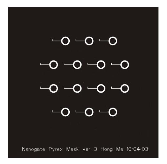
Figure 37: Mask for the Nanogate Pyrex base
