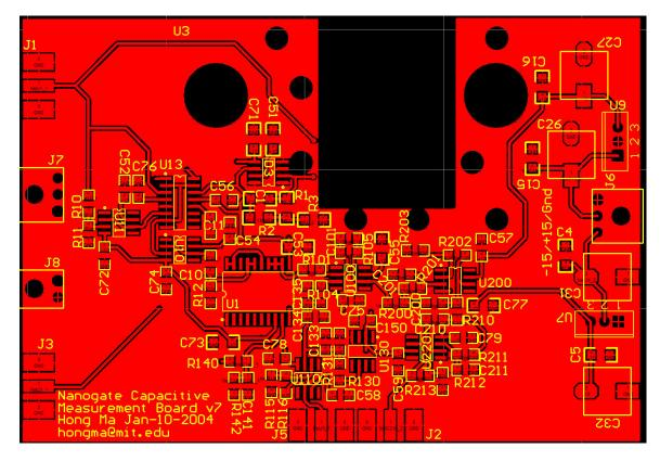
Figure 40: Analog front-end PCB layout, top layer
