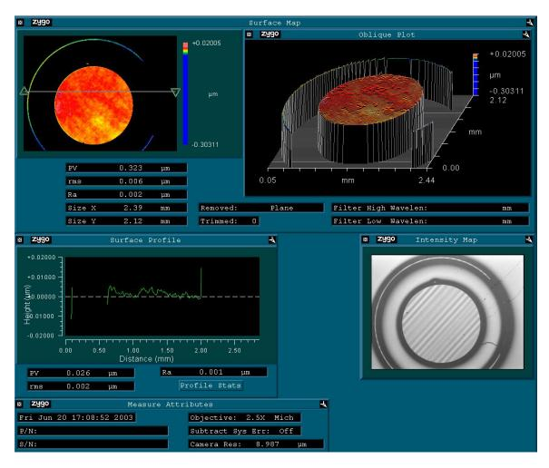
Figure 8: Profilometer scan of the silicon valveland showing 2nm rms surface roughness.
