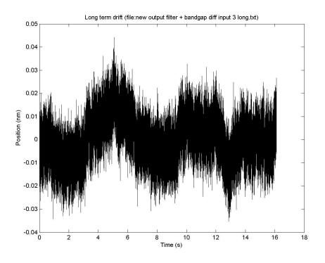
Figure 29: Drift from bandgap reference and output filter
