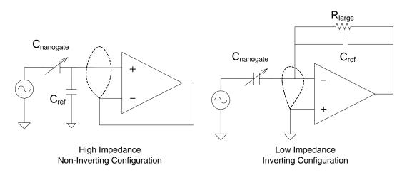
Figure 13: Input amplifier in high and low impedance configuration
