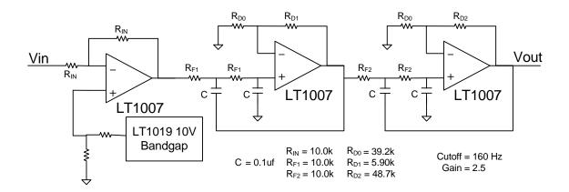
Figure 15: Level shifter and 4-pole VCVS low-pass filter
