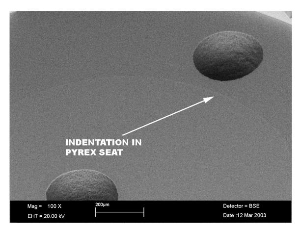
Figure 11: SEM of the Pyrex surface after bonding. The faint circle shows the indentation made by the silicon during the anodic bonding process.
