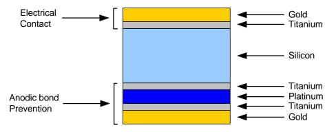
Figure 7: Metal Deposition on Silicon Wafer (not to scale)
