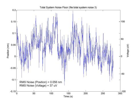
Figure 28: Noise waveform of the full differential capacitive sensing circuit
