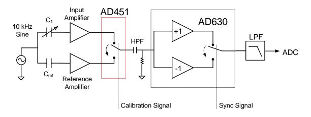
Figure 16: Switched calibration circuit
