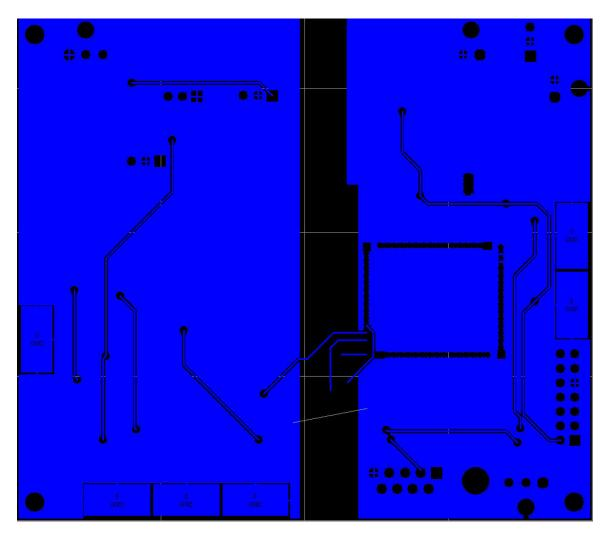
Figure 43: Data acquisition PCB layout, bottom layer
