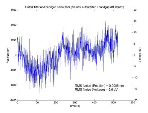
Figure 27: Noise waveform from the output filter and bandgap reference
