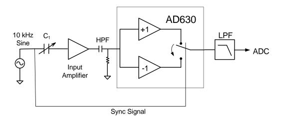
Figure 12: Capacitive sensing front-end
