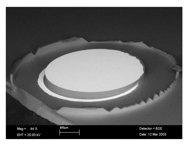
Figure 9: SEM Micrograph of the silicon diaphragm after the fulcrum is deliberately broken from the anodic bond with the Pyrex wafer
