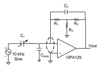
**Figure 14: Input Amplifier Schematic**
