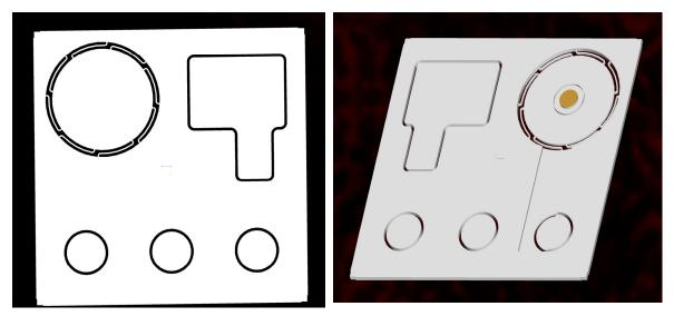
Figure 4: Nanogate die 3D model. Left: topview, Halo's are used to reduce etching time. Right: bottom view, a trench is designed to accommodate the capacitive electrodes on the Pyrex.
