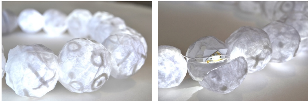
Figure A.14: Jewelry prototypes with illuminated paper-mâché beads with backlit patterns by Yael Freidman. Open bead with exposed LED circuitry inside (lower right).
