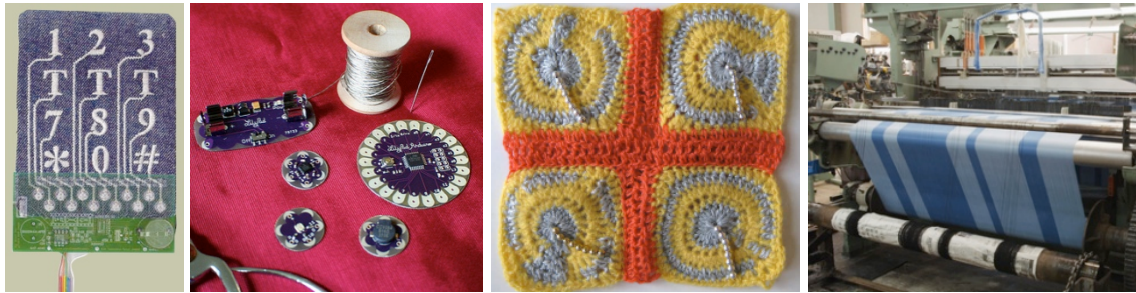
Figure 2.5. From left to right: Embroidered key pad by Post et al., Lilypad Arduino toolkit by Leah Buechley, crocheted tilt sensor by Hannah Perner-Wilson and interactive textile woven on industrial loom by Poupyrev et al.
