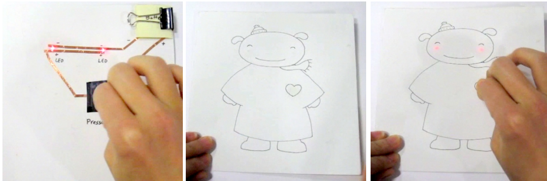
Figure 1.3. Blushing puppy card made with red LEDs and DIY pressure sensor.
