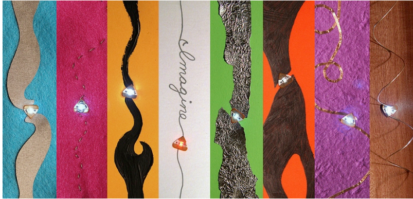
Figure 3.9. Circuits stickers used with a variety of conductive materials including conductive ink, tape, foil, pencil graphite, thread and soldered to wire.
