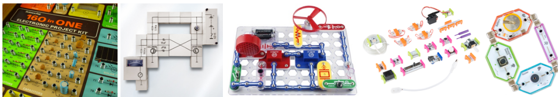
Figure 2.1. From left to right: 160-in-one Science Fair Electronic Project kit with springs as connectors (image by mightyohm); Braun Lectron System, Snap Circuits (image by Adafruit), littleBits (image by Sparkfun Electronics) and LightUp (image from lightup.io 4 ) with magnets as connectors.
