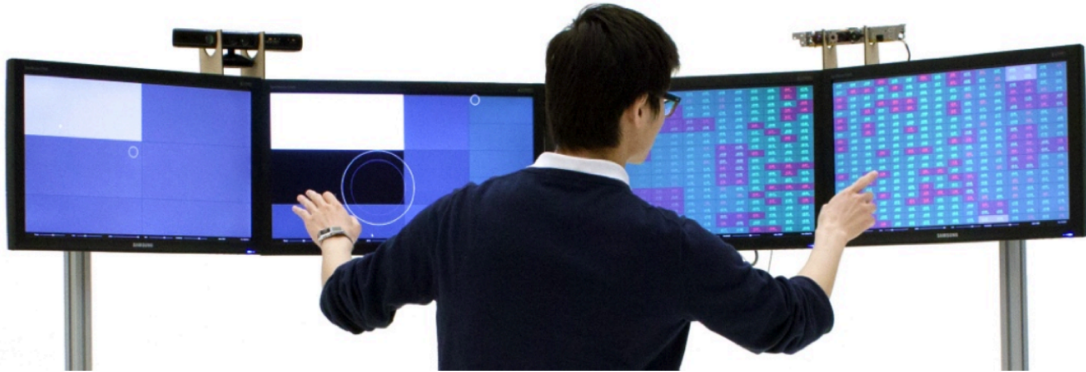
Figure 4-1: The Perifoveal display encodes information into the user's visual periphery that can summon an onlooker's attention
