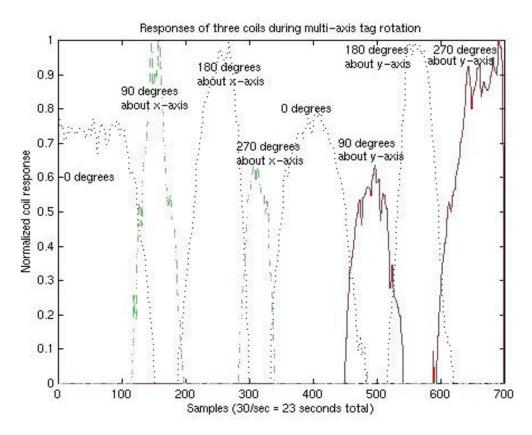
Figure 29. Normalized responses from three coils for one tag during tag rotation around coil axes. As the tag signal decreases along one axis, it increases along another. Labels indicate rotation represented by each graph peak.
