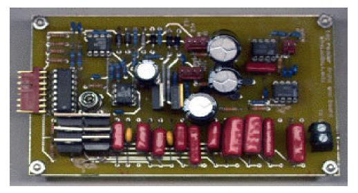
Figure 3. Triac and capacitor ladder board with driver and front-end circuitry.
