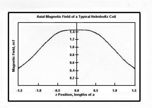
Figure 23. Axial magnetic field of a typical Helmholtz coil, with coils spaced distance *a* apart, where *a* is the radius of a coil.
