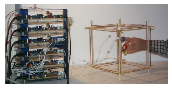
Figure 26. The first completed six-coil cube frame with six tag reader boards.
