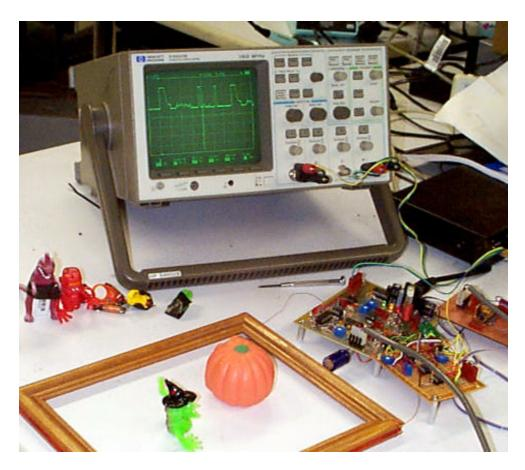
Figure 9. Second prototype of swept-frequency tag reader system.
