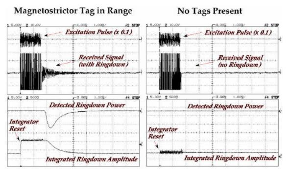
Figure 5. Signals from completed ringdown reader system.
