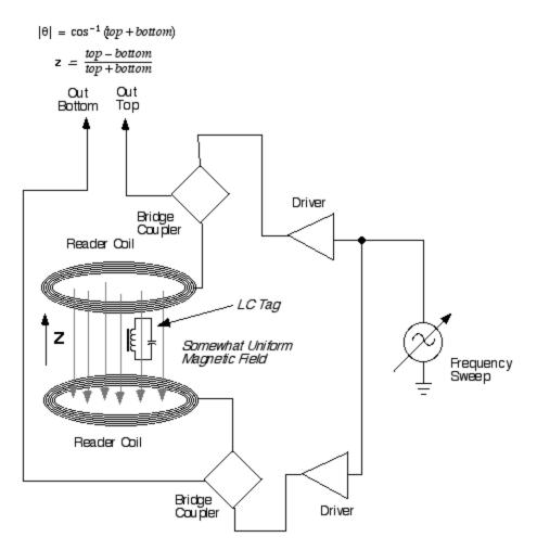
Figure 24. Two-coil Helmholtz arrangement block diagram.
