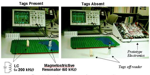
Figure 8. An early prototype swept-frequency tag reader.
