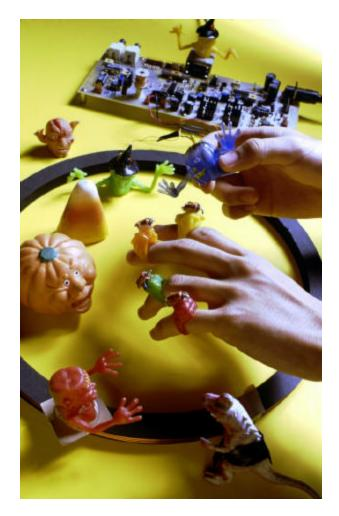
Figure 15. Musical Trinkets, with tag reader, read coil, and objects.
