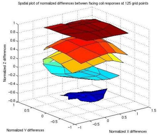
Figure 28. Mesh visualization of raw data from tag readers along an evenly-spaced 5x5x5 grid. Although results were irregular, relative positions were fairly conserved and so a simple fit algorithm could probably provide decent accuracy.
