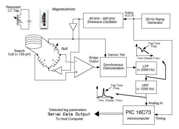
Figure 6. Block diagram of swept-frequency tag reader.
