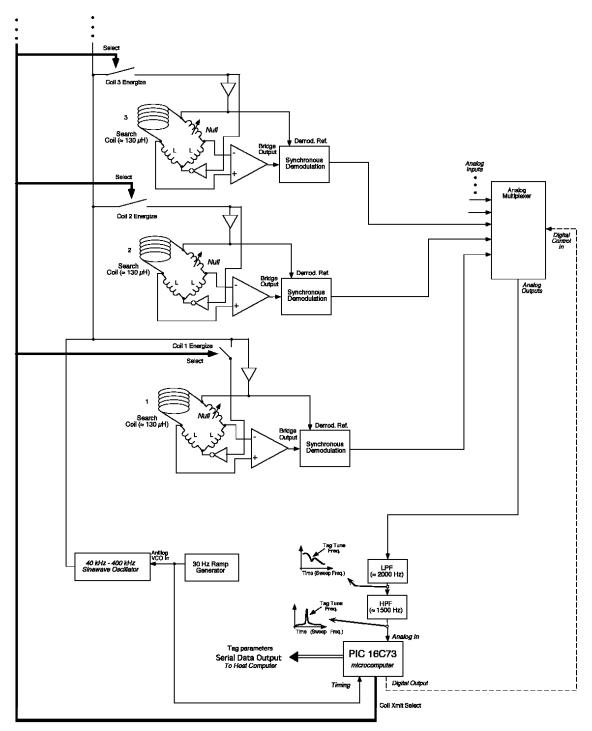
Figure 25. Block diagram of six-coil tag reader system.
