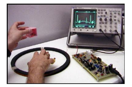
Figure 10. A more mature tag reader. Electronics have been incorporated into a single board, and the ring for the coil was made specifically for this purpose.
