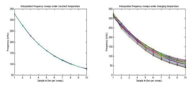
Figure 13. Interpolated frequency curves during single tag-reader sweeps. Left: curves taken during twelve hours of constant temperature, all plotted atop each other. Right: curves taken during ten minutes of temperature change, plotted over each other.
