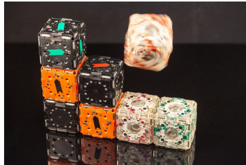
Figure 5-6: One modular robotic cube snaps into place with rest of the M-blocks.
