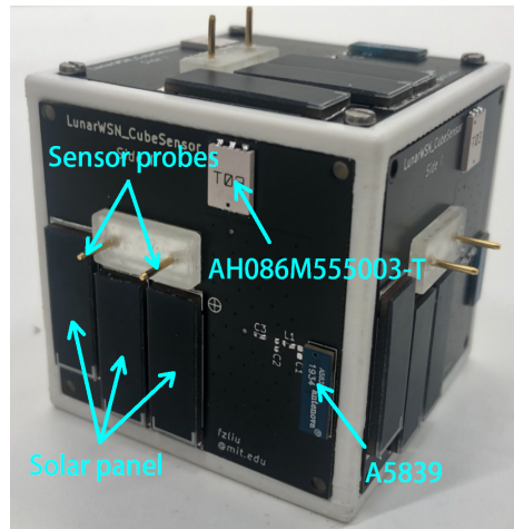
Figure 2-13: The structure of the sensor node side.
