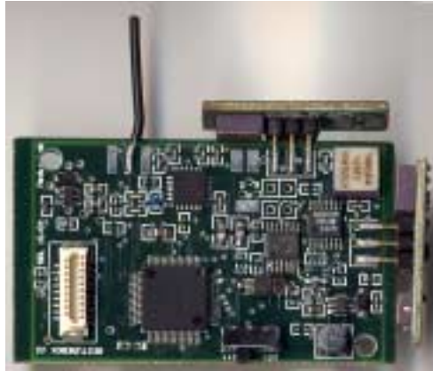
Figure A-4: Front side of main board with daughter boards mounted
