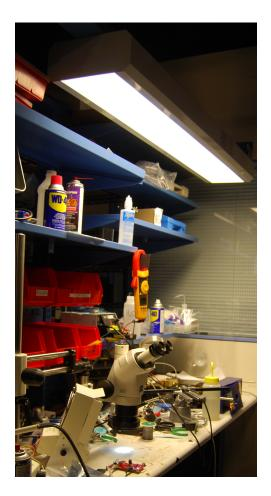
Figure 6-4: The microscope/soldering station workbench with ambient light
