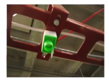
Figure 5-2: A "MERL" [31] movement node mounted on the ceiling
