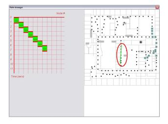
Figure 4-2: Marking the path (green line, circled for clarity in the figure above) that the user wants to detect people walking on. The left pane contains manipulable time data.
