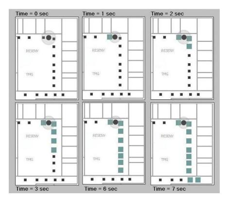
Figure 3-4: "Seeing" a contiguous set of motion sensors detect motion. The six images represent successive time slices with the earliest at the top left and the latest at bottom right. The black icons indicate movement sensors. The icons pop out and change color as they detect motion. Here, it is easy to infer that at least one person is walking underneath (color image).
