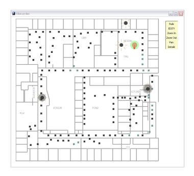
Figure 6-1: Test Setup: Location of nodes. One "Spinner" node was deployed next to the elevator, another in the kitchen. One node was deployed "Resenv" area (Responsive Environments area) near the microscope/soldering station. Another node close the Resenv Area is located within the author's office. The nodes in the public areas (elevator, kitchen), have large halo's (indicative of high sound levels). The nodes deployed in the Resenv area report low sound levels.
