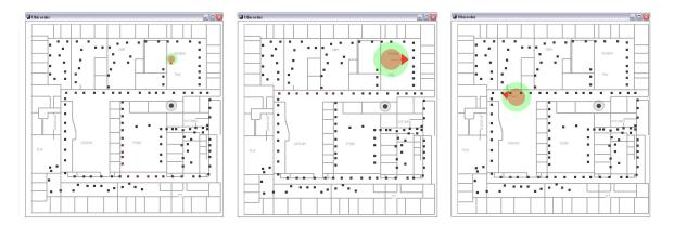
Figure 3-7: The green and red circular icon represents user's location. The icon's arrow indicates orientation, and the size of the icon changes with the localization accuracy.
