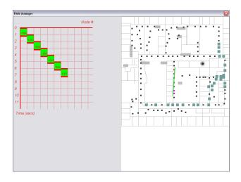
Figure 4-3: Nodes changing color in the order of the drawn path, indicates the direction of walking that will be detected, and the time between which adjacent nodes must detect motion.
