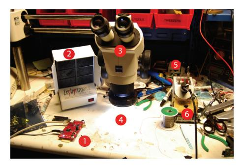
Figure 6-5: Zoomed in view of the Spinner Node deployed on the microscope/soldering workbench. (1) Spinner Node, (2) fume exhaust, a device incorporating a fan and a filter to absorb noxious solder fumes, (3) microscope, (4) Area under the microscope, illuminated by a LED spotlight, (5) LED spotlight switch, (6) Soldering Iron
