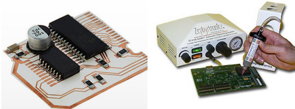
Figure 3.3 Component attachment with low-temperature solder paste and a solder paste dispenser.
