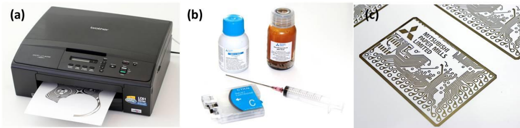
Figure 3.2 Conductive Inkjet printing with off-the-shelf printing and conductive silver particle ink. (a) An example inkjet printer with silver nano particle filled ink cartridges. (b) Silver nano ink and replacement ink cartridges. (c) Example printout from Mitsubishi paper mills limited.
