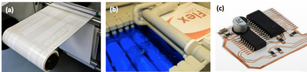
Figure 3.1 CIT printing technology with 2 stage additive process. (a) Stage 1, inkjet printing (360 dpi) with onboard UV and IR curing. (b) Stage 2 - electro-less copper plating. (c) Example flexible circuit with copper traces on Mylar substrate.
