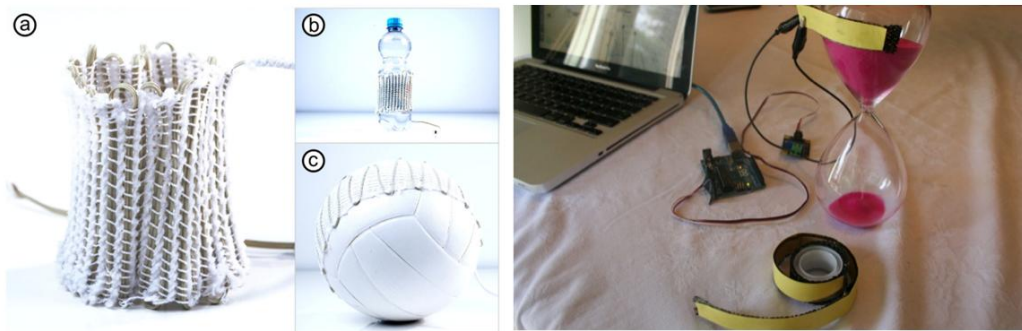
Figure 2.4 Left: Modular and Deformable Touch-Sensitive Surfaces Based on Time Domain Reflectometry. Right: TactileTape: low-cost touch sensing on curved surfaces.
