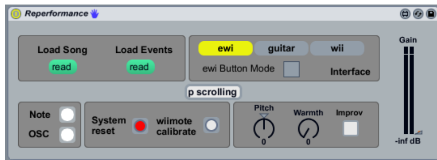
Figure 3-16: The primary user interface for Expressive Re-performance. It includes buttons for opening audio and analysis files, selecting instruments and EWI performance mode, resetting the song, calibrating the Wii and visual feedback on expressive input and data inflow. Double clicking on the scroll patch will bring up the visual progress reference.
