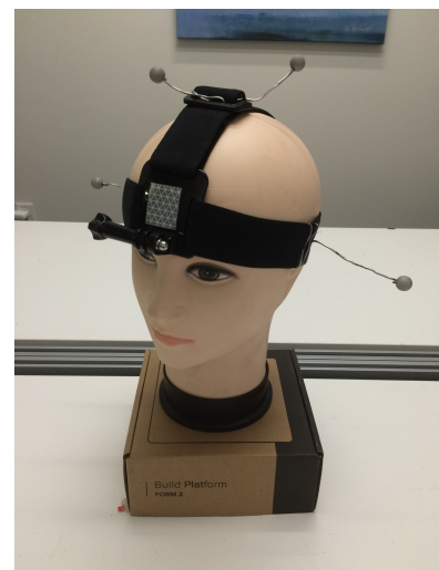
Figure 22: Optical markers placed on the user’s head for tracking
