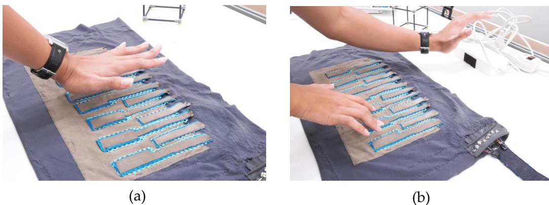
Figure 7.12: Non-contact gestures a) proximity b) e-field sensing by waving towards a source
