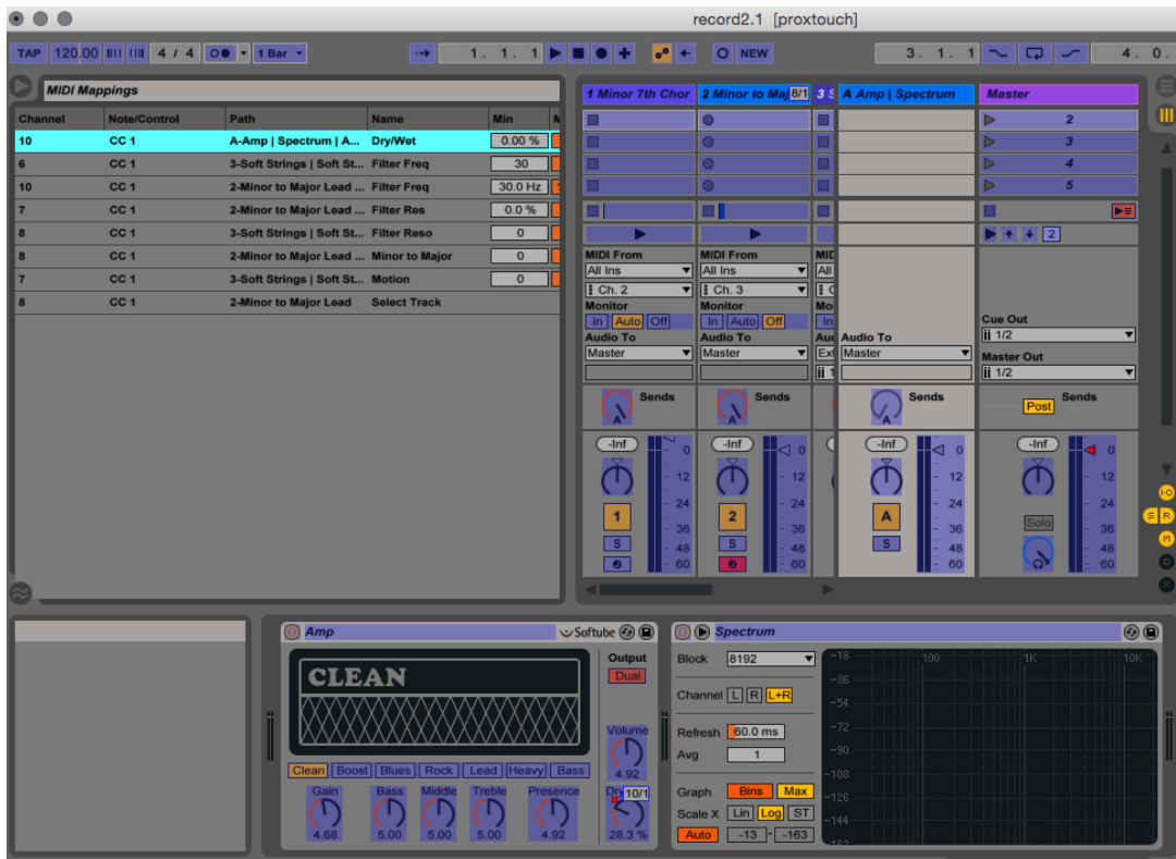
Figure 6.6: In this MIDI parameter mapping panel, we can see all of the MIDI channels currently used and its corresponding Path/Controls. Parameter mapping can be done by pressing any available control (shown in purple) and correlating it to a MIDI message (by triggering the controller).
