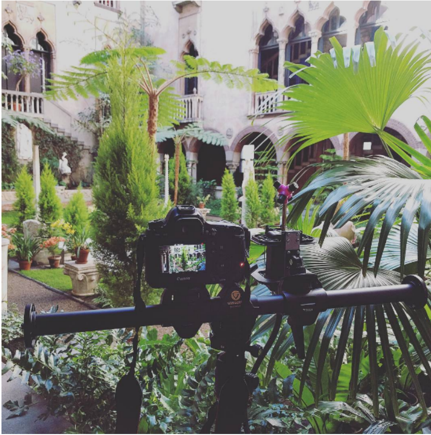
Figure 1: The recording setup, including a camera and a tetrahedral microphone, in the Isabella Stewart Gardner museum
