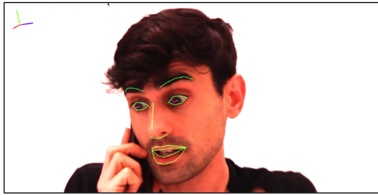
Figure 12: Facial feature points, head and pupil orientation extracted by the Intraface code library.
