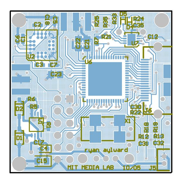
Figure A-8: Node main board layout, bottom layer.
