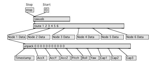
Figure E-1: Patch showing rawusb external used to extract data from the USB basestation.
