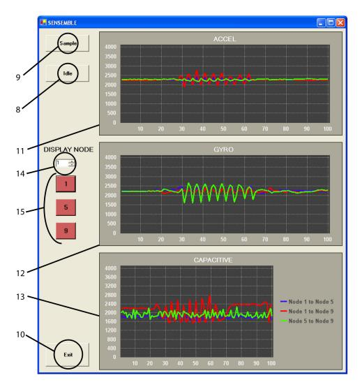
Figure 4-3: User interface for visualizing sensor data in real-time.
