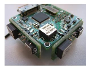
Figure 2-5: Orthogonal mounting of sensor daughtercards.
