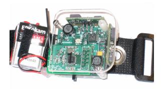
(a) Fully assembled sensor node.
