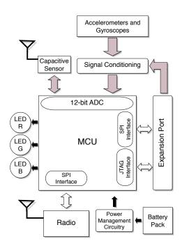
Figure 2-2: Sensor node architecture.
