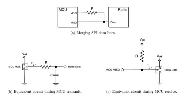
Figure 2-10: Modified SPI interface for Nordic radio.
