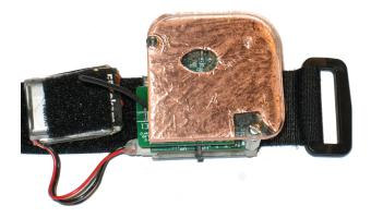
Figure 6-2: Faceplate electrode for capacitive sensor.
