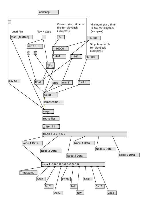
Figure E-3: Patch showing usage of  $\mathtt{seq}\sim$  for loading and playing back data from a text file.
