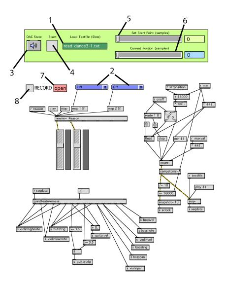
Figure E-5: Interface for streaming recorded text files Into Max/MSP.
