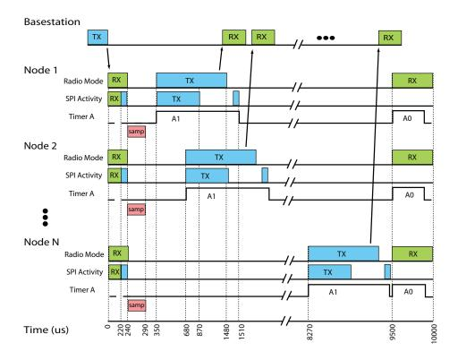
Figure 3-2: Detail of network timing cycle.
