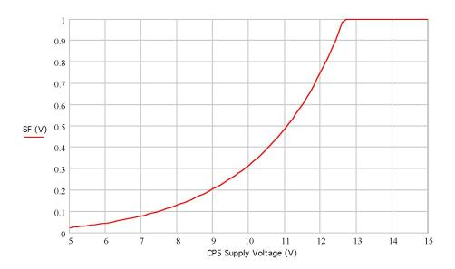
Figure 7-2: Relative scale factor of sensitivity versus driving voltage for the ADXRS300 gyroscope.
