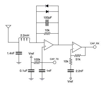
Figure 2-6: Capacitive transceiver circuit.
