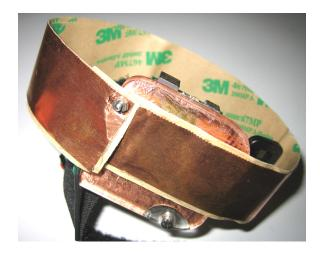
Figure 6-1: Bracelet electrode for capacitive sensor.
