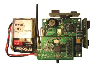
Figure 2-3: Assembled node board and battery pack.
