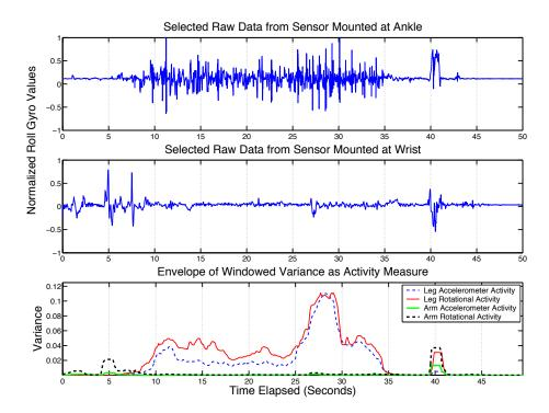
Figure 5-5: Selected data and resulting activity envelopes as dancer transitions from slow kicks to rapid tense kicks. Sequence of leg motions is framed by stylistic arm motion.
