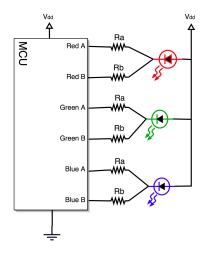
Figure 2-9: Resistor network for controlling the RGB LED.
