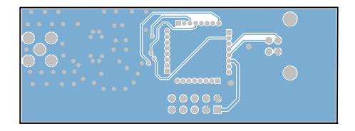
Figure A-14: Basestation layout, bottom layer.
