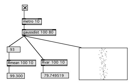
Figure E-2: Externals Rmean and Rvar usage.
