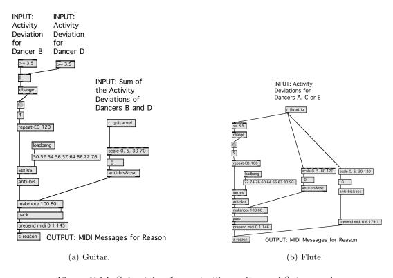
Figure E-14: Subpatches for controlling guitar and flute sounds.
