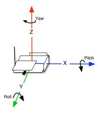
Figure 2-11: Axis conventions for inertial sensor data.
