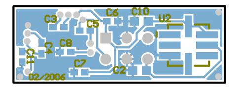
Figure A-16: High range sensor card layout, bottom layer.
