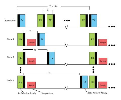
Figure 3-1: Basic illustration of the TDMA communications cycle.
