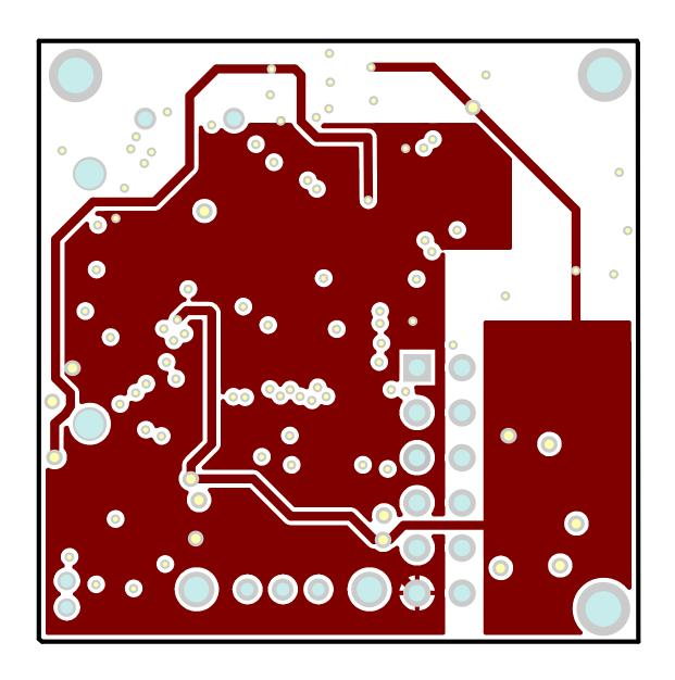
Figure A-7: Node main board layout, internal layer.
