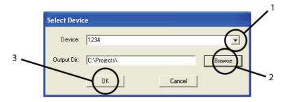
Figure 4-1: Select form user interface for connecting to the USB device.
