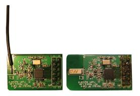
Figure 2-12: RF daughtercards comparing wire antenna to chip antenna.
