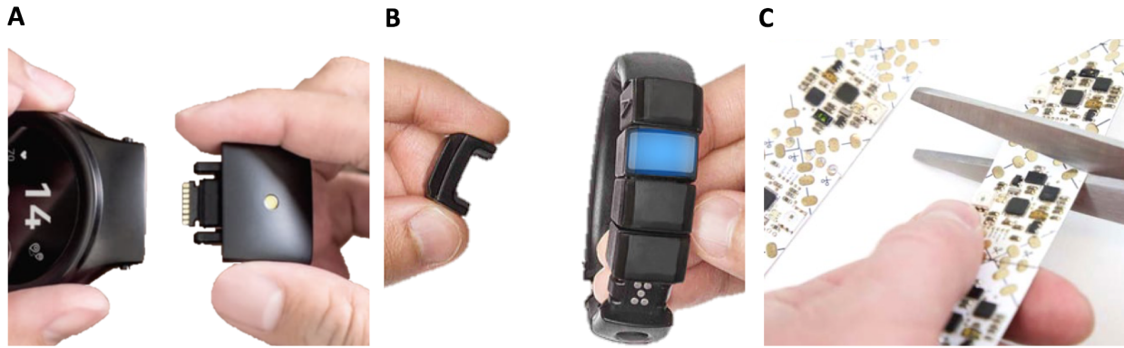
Figure 3: Modularity in commercial wearable devices. A) BLOCKS smartwatch, commercially available for $259 [16]. B) Nex Band, a modular smartband that has evolved into a non modular band in their first commercial release [17]. C) SensorTape, a modular flexible dense sensor network [18]
