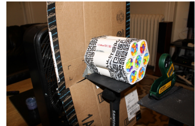
Figure 19: A picture of a simple laminar flow test setup for rough wind directivity characterization
