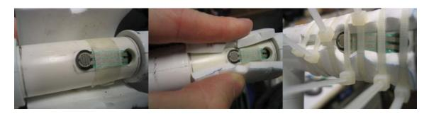
Figure 2-9: How the upper handle's FSR was attached and surrounded with foam
