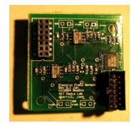
Figure 2-15: The Electric Field Sensing layer
