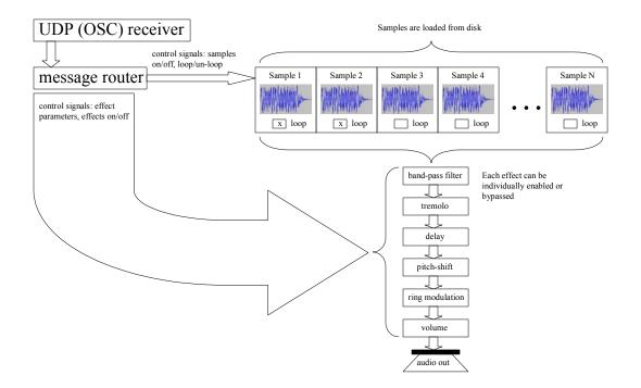
Figure 3-12: Control data (left) and audio (right) flow in the pure-data patch.
