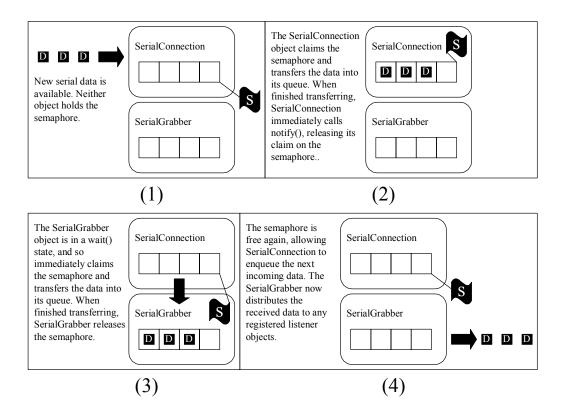
Figure 3-5: Semaphore-based serial data handling
