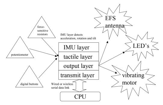
Figure 2-4: Overview of stack configuration used for the device 2.3 Application-specific circuits
