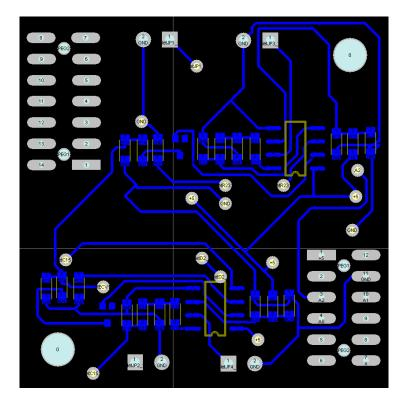
Figure B-7: PCB for the Electric Field Sensing Layer top (top), and bottom (bottom)
