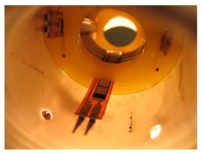
Figure 2-14: Bend sensors mounted inside the right hand handle.
