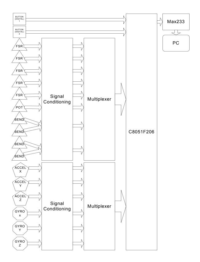
Figure 2-17: Hardware system data-capture overview
