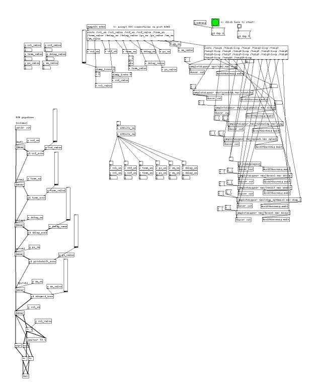
Figure F-1: The main Pure-Data patch for sound triggering and modification
