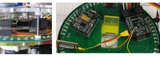
Figure 2-2: Close-up of transmit (top) and tactile (bottom) layers.
