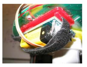
Figure 2-13: The power layer attaches to the bottom of the main body.
