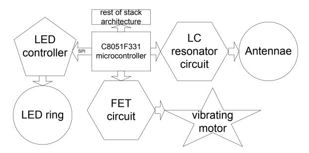
Figure 2-5: Hardware overview for the output layer
