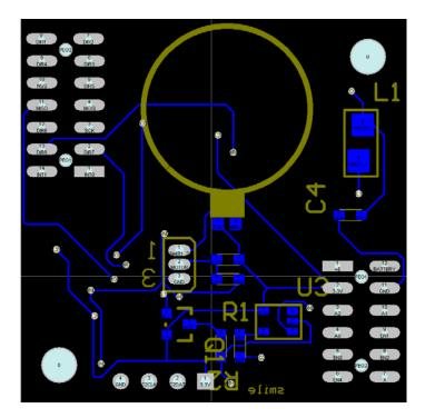
Figure B-2: PCB for Output Layer top (top) and bottom (bottom)
