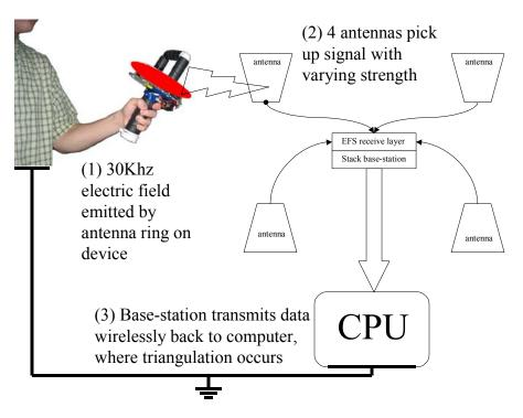
Figure 2-16: Electric Field Sensing setup
