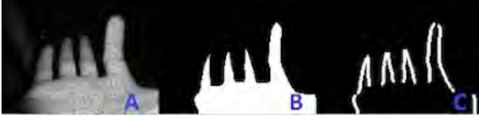
Figure 4-3: Image A shows the raw amplitude image returned by the TOF camera. B shows the thresholded image, and C shows the vertical edges returned by the Sobel derivative filter in the horizontal direction.
