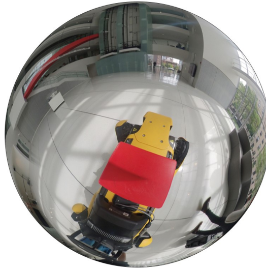
Figure 4-10: A 360° photo captured by the Insta360 ONE X VR camera mounted on Spot that offers a panoramic perspective. With its wide 360° horizontal FoV and 180° vertical FoV, this image provides a comprehensive and immersive view of Spot’s surroundings at the E14 Building of the MIT Media Lab.
