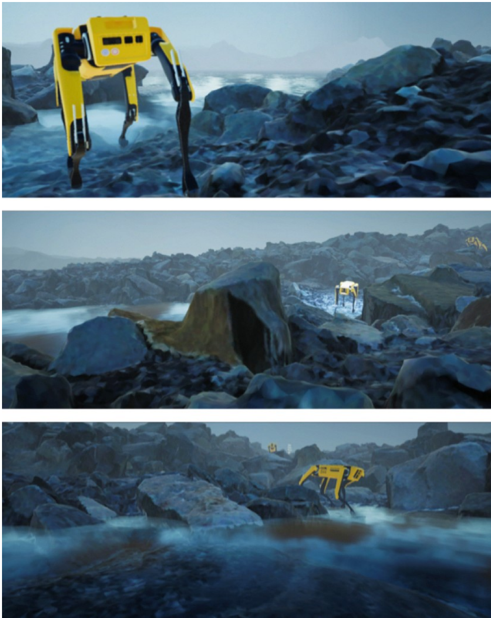
Figure 4-9: Images of the simulated Spot as it navigates a virtual analog site. The terrain is generated using a blend of high resolution aerial imaging based photogrammetry as well as other high resolution 3D assets, providing an immersive and realistic simulation. For a more detailed exploration of the terrain generation process, refer to the comprehensive insights outlined in Chapter 5.
