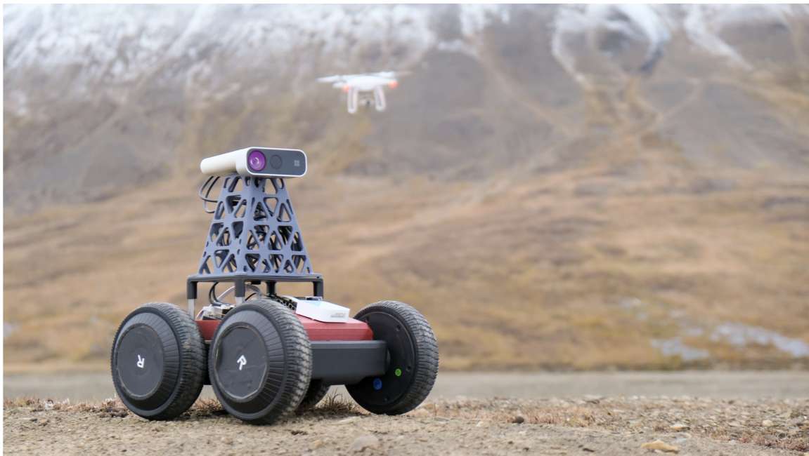
Figure 5-4: Collaboration between terrestrial and aerial unmanned vehicles for data collection purposes. The Microsoft Azure Kinect is integrated as a custom payload atop the Rover Mini body. This dynamic setup, detailed in Chapter 3, empowers the rover with depth data collection capabilities. As the Rover Mini traverses the field sites, the Azure Kinect captures high resolution ground-view scenes for precise 3D reconstruction, while the DJI Phantom drone soars above, to capture larger terrains. Image Courtesy of Maggie Coblentz.
