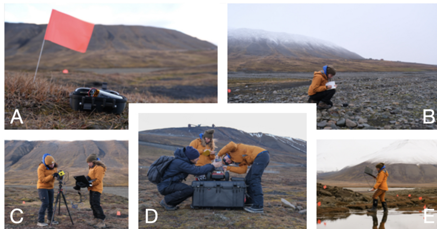
Figure 5-5: Image A - Arduino environmental sensor in custom hard-shell case. Image B and C- C. Paige collecting field notes, C. Paige collecting data using the Microsoft Azure Kinect, C. Paige, S. Image D - Auffinger and J. Todd preparing a mini rover with the Microsoft Azure Kinect mounted on a custom payload tower for data collection. Image E - C. Paige and J. Todd collecting data using a Velodyne puck on a custom 360° rotating mount (collection for a separate project, Ward et al., at ICES 2023) [190].
