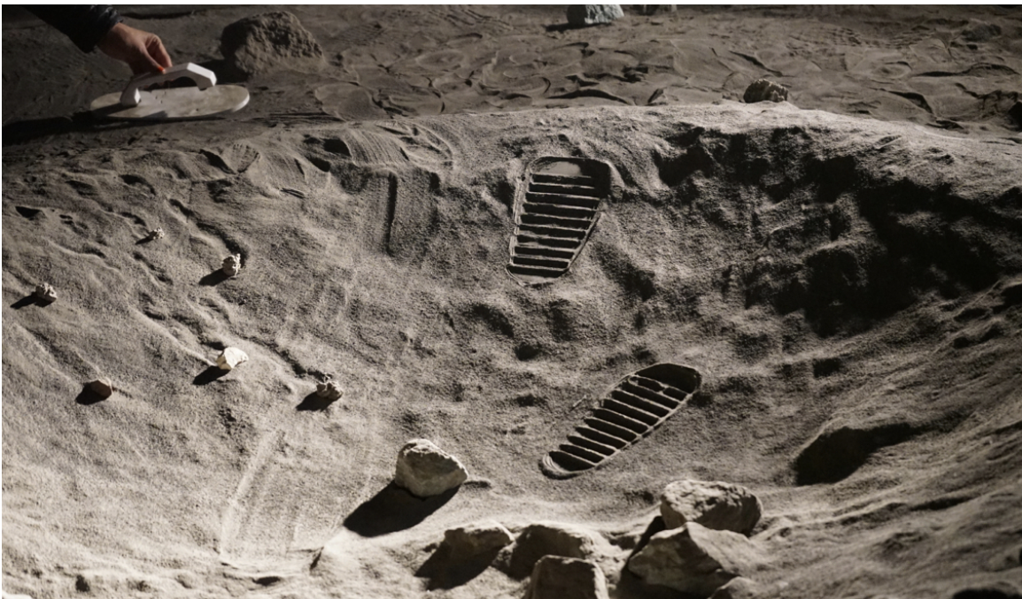
Figure 6-15: This captivating image showcases the intricate detail of 3D printed soles designed to replicate the footprints left by astronauts during extravehicular activities (EVAs). These custom soles faithfully recreate the distinctive patterns and textures of the original boot imprints, allowing for a precise and accurate representation of the astronaut's footsteps. Image courtesy: Cody Paige and Ferrous Ward.
