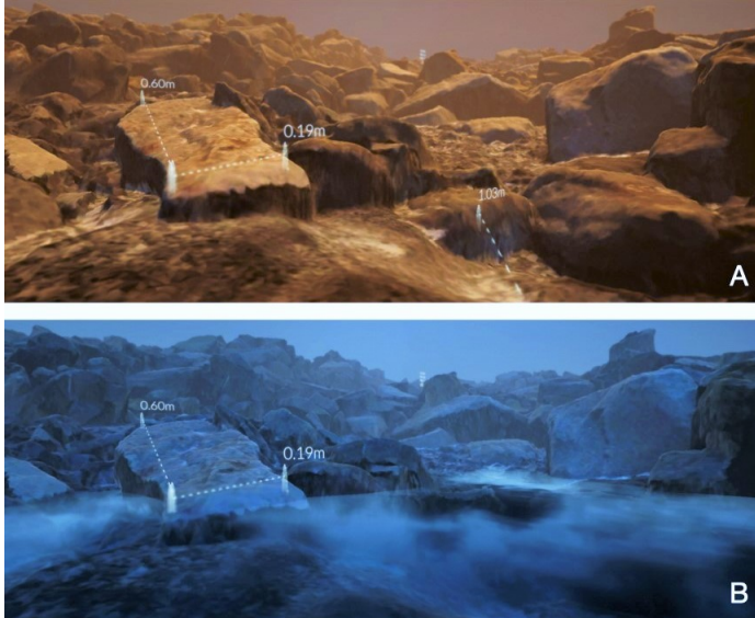
Figure 5-15: Two images highlighting the measurement tool integrated into the virtual environment, allowing users to explore, annotate, and extract precise measurements. In addition, the analog site filter removes certain high-resolution assets, such as water meshes, providing a direct comparison between the analog and real environments. Image A showcases the analog site, while Image B reveals the corresponding real site, offering a comprehensive understanding of the virtual representation and its real-world counterpart.
