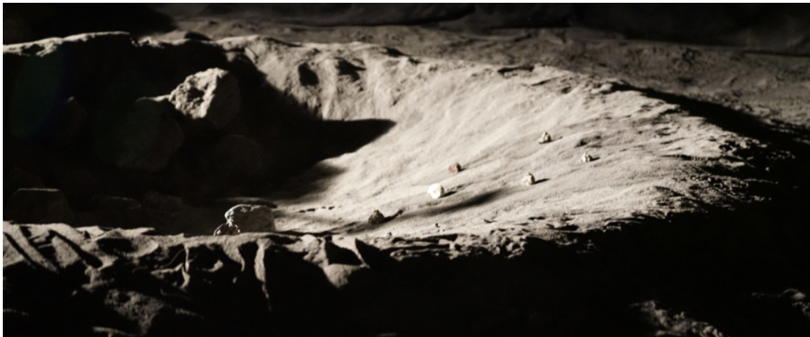
Figure 6-10: NASA Ames Research Center SSERVI Testbed a sandbox of simulated regolith for lunar studies. Image courtesy: Ferrous Ward.
