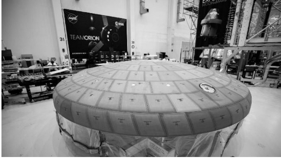
Figure 1-14: HoloLens 2 devices assisted technicians during the manufacturing process for the Artemis II heat shield. One of the most critical elements of Orion, it protects the capsule and crew during reentry through Earth's atmosphere.
