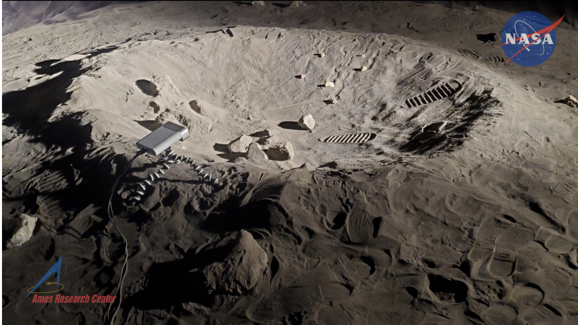
Figure 6-11: A view of the NASA Ames regolith test bed featuring the Azure Kinect camera during its testing phase. This image provides a real-world representation of the camera's deployment in a lunar analog environment
