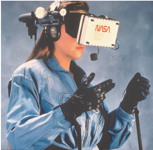
Figure 1-11: Pioneering the realm of Virtual Reality, NASA Ames, in collaboration with VPL Research, Inc., unveiled the Virtual Interface Environment Workstation (VIEW) in 1990. The stereoscopic head-mounted display system allowed users to immerse themselves in computer-generated or real environments captured from remote video cameras. The DataGlove, adorned with fiber optic cables and sensors [40], faithfully translated finger movements into the virtual world, enabling users to interact with computer-generated objects.
