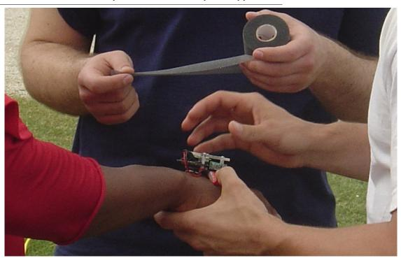
The forearm and upper arm received a similar treatment, however without the stim pad. The chest node was attached using a Polar heart rate monitoring strap that received the same hook velcro as the stim pad. A prewrapped arm and the chest strap are visible in FIGURE 7-61.
