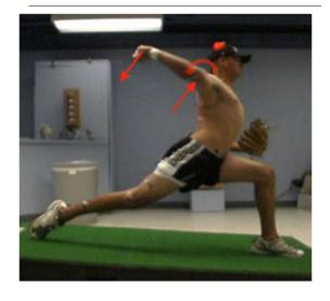
The parameters *imuPeakDistract* and *optPeakDistract* are the mean peak distraction values over all pitches for each pitcher. For the IMU system, Pitcher 2 has an average distraction force of 798.7N while the average optical system distraction force is 509.1N; this is a difference of 36%. For Pitcher 1, the average IMU distraction force is 2888.2N and the average optical distraction force is 636.0N, this is a difference of 78%.
