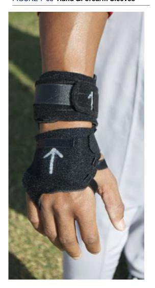
In order to secure the nodes, sleeves and straps into place on body segments, hook velcro was sewn into place.
