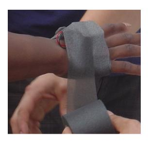
attempt was that too much time was (10-15 minutes) spent instrumenting the player, which impeded their workflow, and application directly to the skin, even with pre-wrap, caused failures when sweat began to short out the inertial nodes.
