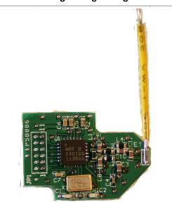
FIGURE 4-23 nRF2401 Based Wireless **Expansion Board**
