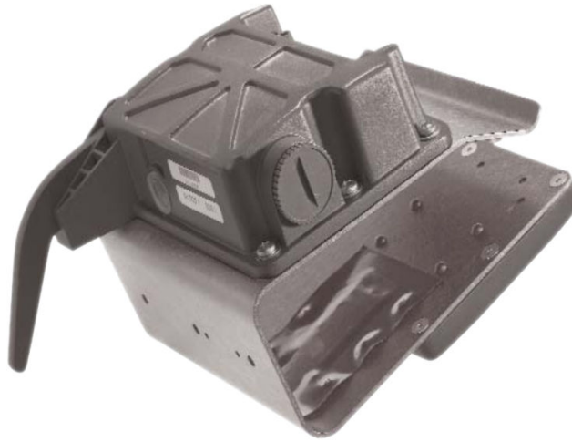
Figure 1.1: The Savi Technology ST-676 tag mounts onto container doors [55].
