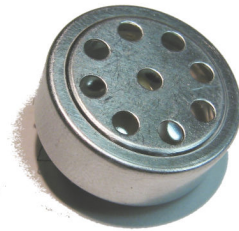
Figure 2.18: A piezoelectric microphone can wake the microcontroller on loud sounds.
