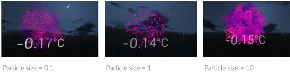
Figure 29. An experiment to increase the particle size as a method to increase visibility, but decrease computation expense. Ultimately, the particle size was increased slightly, but the very large particle sizes caused a loss in the larger systematic pattern of movement.
