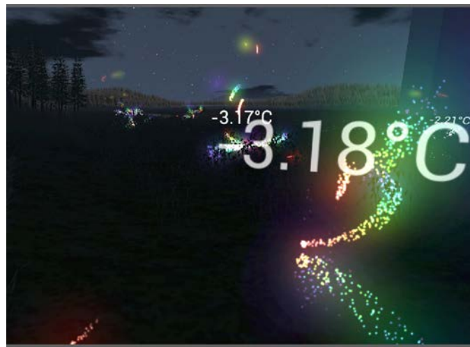
Figure 17. An early test to automatically generate a particle system at the site of each sensor node when the node subscribes and then update when the data changes.
