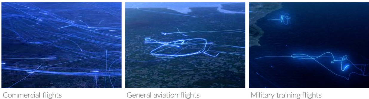
Figure 9. Stills from UK National Air Traffic Services visualization of flights at Heathrow airport on a typical day [35]. Three-dimensional motion path signatures clearly distinguish the different types of flights.
