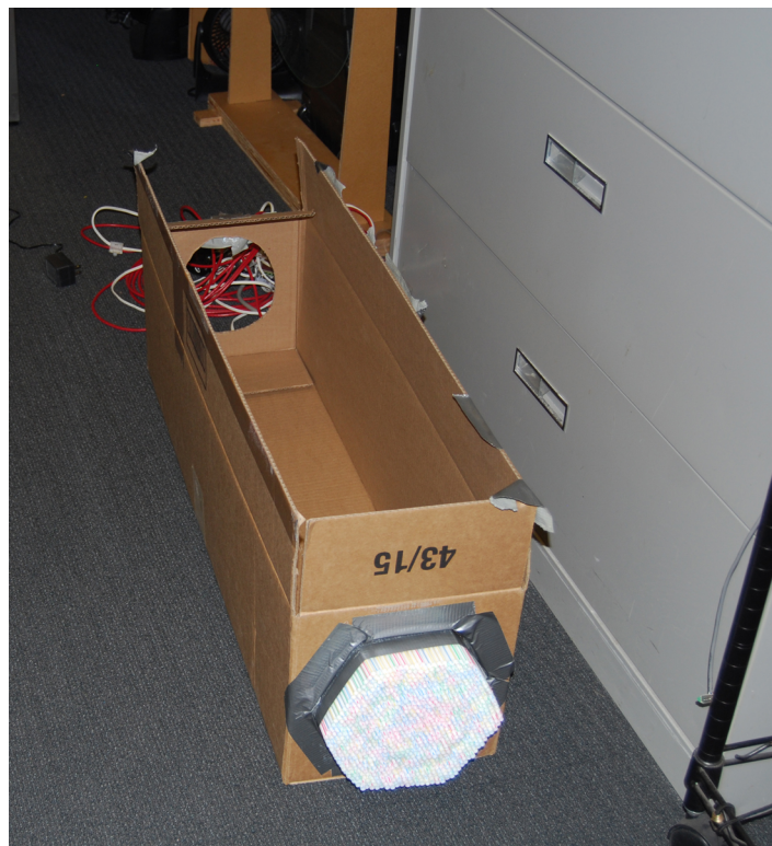
Figure 3.3: Constructed wind tunnel.
