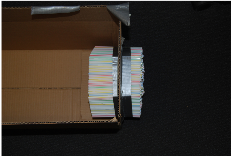
Figure 3.2: Flow straightener honeycomb for wind tunnel.
