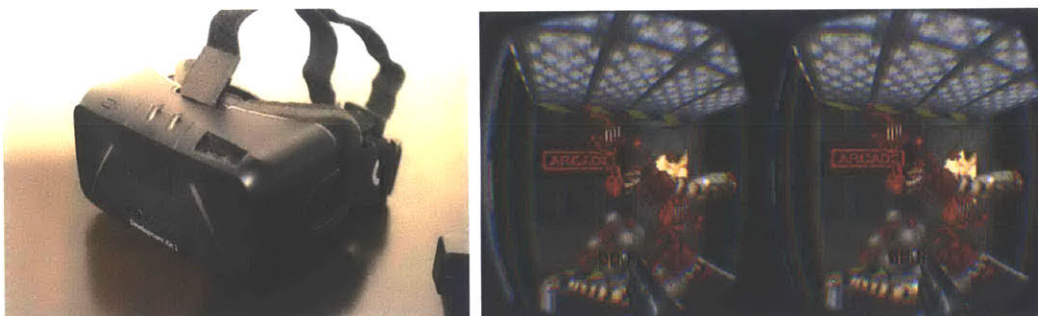
FIGURE 5-9: LEFT: OCULUS RIFT DK2, RIGHT PRE-DISTORTED IMAGES FOR LEFT/RIGHT OBJECTIVES
