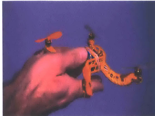
NIXIE, WRIST-WEARABLE QUADROTOR W/CAM
