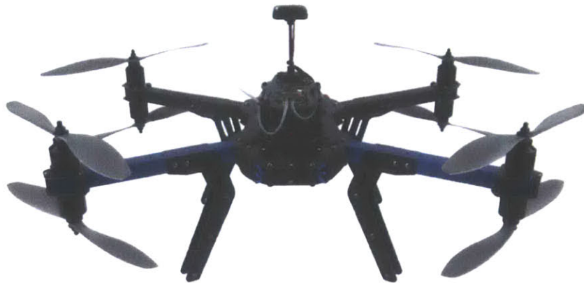
FIGURE 5-2: EIGHT ROTOR X8+ UAV SELECTED FOR USE IN QUADRASENSE [3DR]
