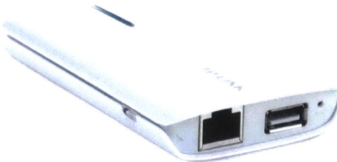
FIGURE 5-6: TPLINK ROUTER SELECTED FOR QUADRASENSE, USB2.0 HS + LITHIUM-ION BATTERY [TPLINK]
