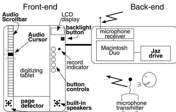
Fig. 3: Components of the version 2 prototype. Design changes from version 1 are shown in bold.
