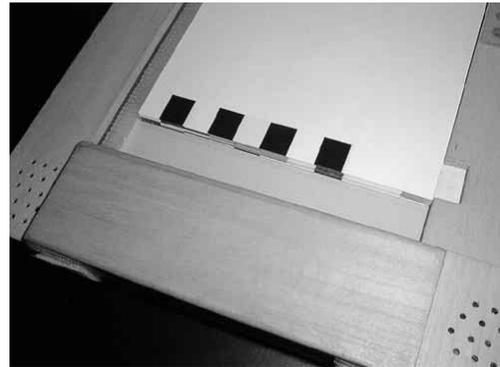
Fig. 4: Both notepad and page numbers are coded on each page. Sensors underneath a hand rest read the code.
