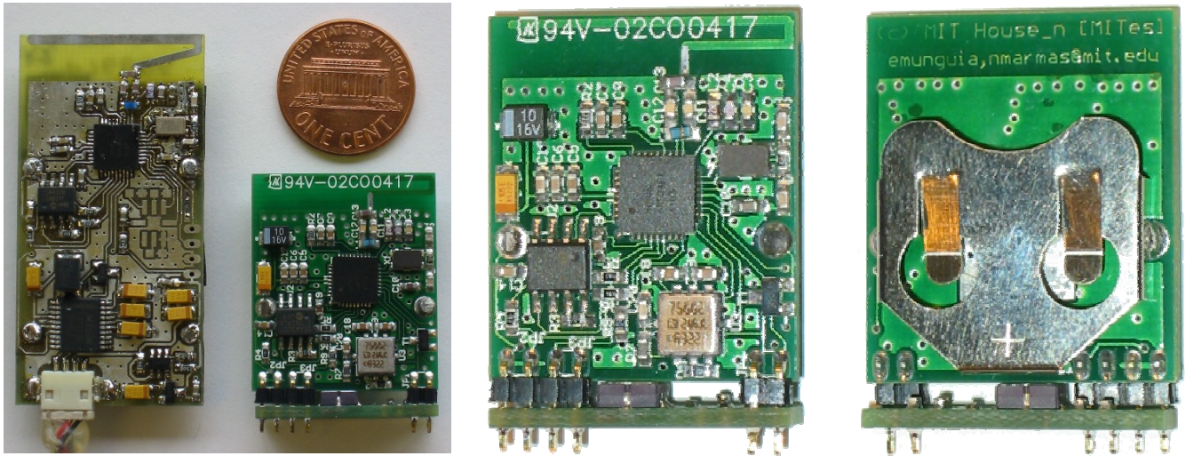
Fig. 3.13 Accelerometers. The receiver (left) is connected to the serial port of the iPaq. Wireless transmitters (middle and right images show front and back) can be placed on different locations of the body. Dimension: 1.2 x 1.0 x 0.25 in. Weight: 8.1 grams with battery.
