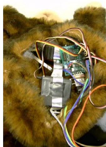
Figure 3-2. Monkey body open, exposing servos, rods and microcontroller board inside.
