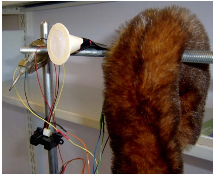
Figure 3-10. Motion and proximity sensors affixed to the monkey stand, from which the monkey is also hanging by its tail. The motion sensor has a cone-shaped Fresnel lens around it.
