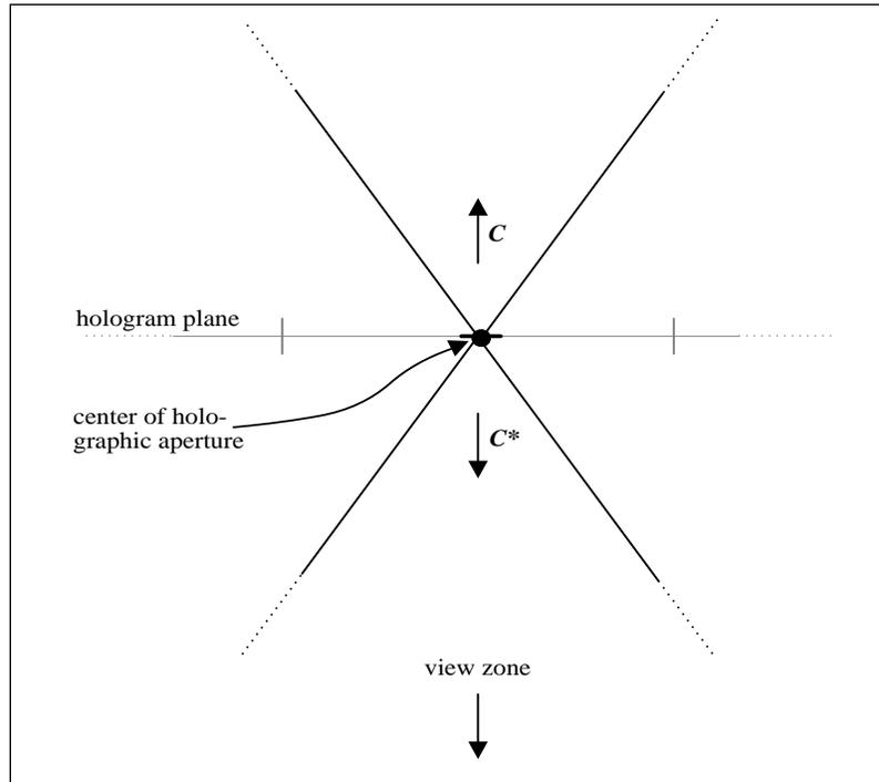
Figure 4. A two-dimensional representation of the two pieces of the double frustum camera. The orthoscopic camera is called  $C$ , the pseudoscopic camera is referred to as  $C^*$ .
