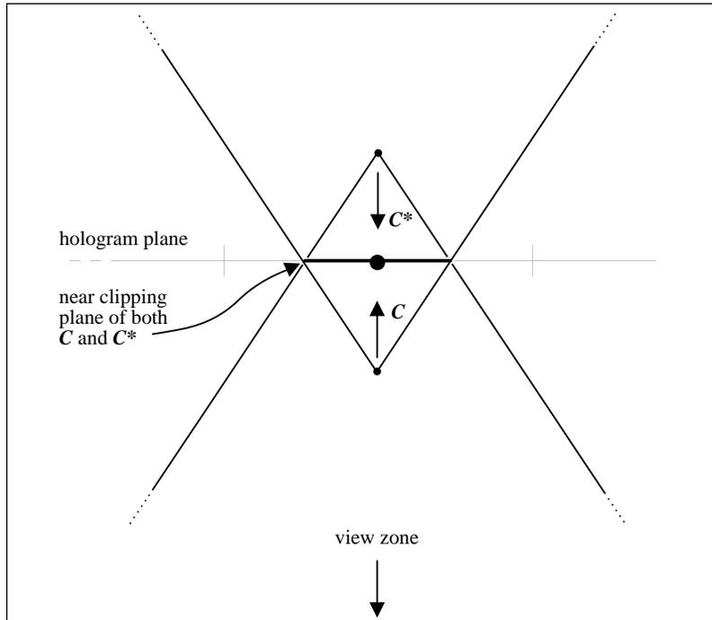
Figure 5. Computer graphics camera geometries have a near plane located a non-zero distance away from the camera position. C and C\* must be positioned so that their near planes overlap at the aperture plane; otherwise, parts of the scene will be imaged twice or not at all.
