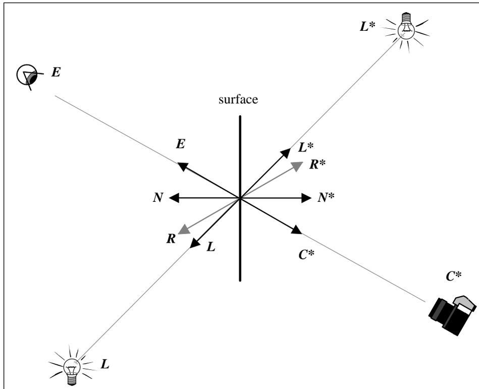
Figure 3. The standard computer graphics relationship between the eye vector  $E$ , the surface orientation vector  $N$ , and the light source vector  $L$  is mathematically equivalent to that between the pseudoscopic camera's vector  $C^*$ , the automatically-flipped normal vector  $N^*$ , and the manually flipped light source vector  $L^*$ .
