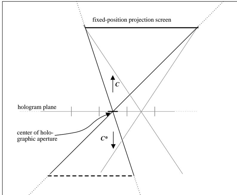
Figure 6. Holographic exposure geometries that use a projection screen fixed with respect to the hologram plane require the double frustum to be sheared to recenter the projection screen area. Cameras  $C$  and  $C^*$  are sheared in opposite directions with respect to the the hologram plane.
