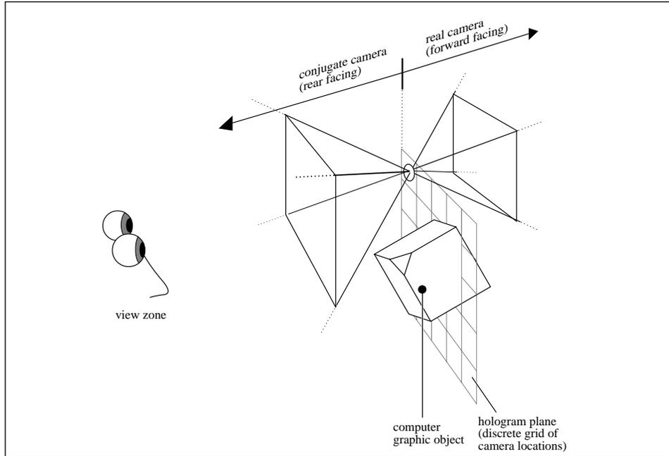
Figure 2. The frustum of a camera used to capture image data for a single holographic aperture of a full parallax display crosses itself at the aperture plane. Since common computer graphics algorithms do not allow a camera with such a frustum, the needed image must be synthesized by using two different cameras.
