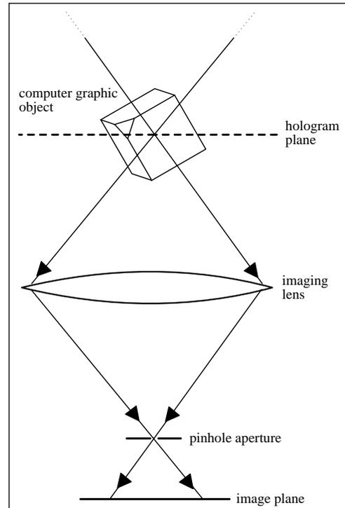
Figure 1. A large imaging lens can be used to move the effective aperture of a pinhole camera into the middle of a scene. A modified camera such as this one can correctly capture image information about parts located both in front and behind the aperture.
