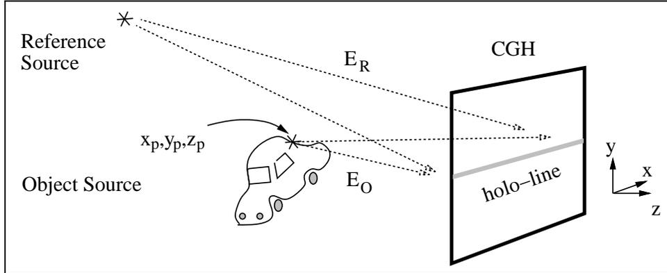
Figure 1: General geometry for HPO CGH.
