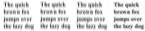
Figure 18: Blurred images used for the subjective evaluation. The shown images correspond to vertical object motion captured with static, coded exposure, motion-invariant, and circular motion cameras (from left to right). All of the six pairs of these four images were presented to the subjects.
