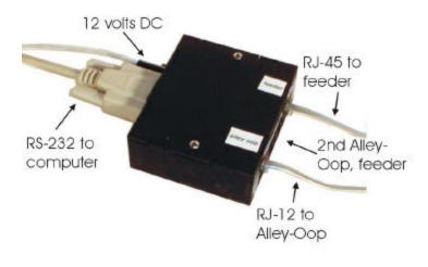
Figure 10-2: Junction box between the dog's computer and the Rover@Home peripherals. All cables are low voltage and present no danger to the dog. The cables to the Rover@Home peripherals are standard crossover telephone RJ-12 cables, easily replaceable from a wide range of vendors such as Radio Shack.
