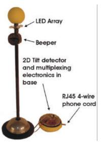
Figure 4-7: Alley oop instrumented to overcome issues of latency, badwidth, and luring. LEDs and beeper can be remotely activated to attract dog's attention, tilt sensors in base detect motion.
