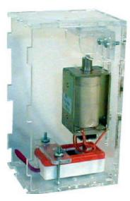
Figure 6-2: The mechanical clicker originally used in Rover@Home. The solenoid presses down on the orange clicker. Because of the different resonance of the box, this clicker sounded different than when held by a user's hand. For this, as well as reasons of simplicity, we decided to instead render the clicker sound through the PC Speaker.
