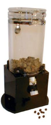
Figure 10-3: Closeup of the custom designed feeder. The top is a 4" diameter x 12" high acrylic canister. The bottom is sawed off and attached to the base with four sheetmetal screws. The screws protrude into the canister and stir the food as the rotator turns, preventing food from simply turning with the rotator.
