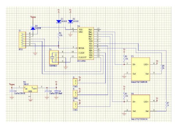
*Figure 11-3: Alley-oop schematic. The ball-tilt sensors on the right are custom made tilt sensors described in section 10.1.3*
