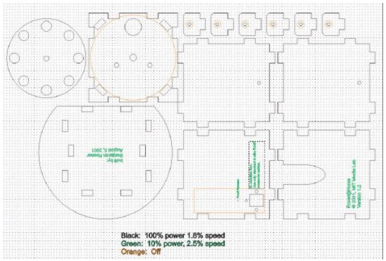
Figure 11-5: Lasercut of the feeder enclosure. Enclosure is made of <sup>1</sup>/<sub>4</sub>" acrylic.
