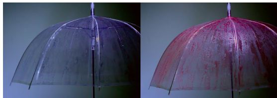
Figure 27. Before and after image of umbrella utilizing Organic Primitives for acid rain sensing and display.
