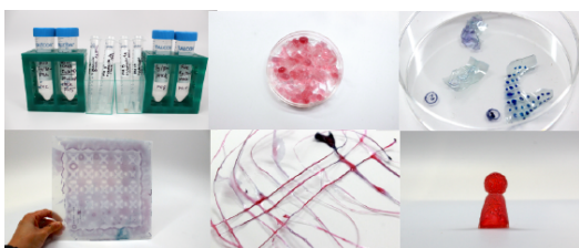
Figure 13. (left to right clockwise) liquid based Organic Primitives ; odor-color changing gel; color-shape changing films; color changing 3D form; odor-color changing fiber; odor-color-shape changing sheets.
