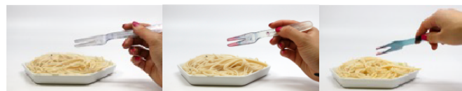
Figure 21. Prototype of utensils at varying levels of degradability. (right) Fully edible and biodegradable utensil. (left) Before and after image of dip-coated, 3D-printed fluidic utensil.
