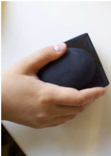
Figure 51: The input side of Honey I'm Home is a small, smooth, black box, designed to sit unobtrusively on the desktop and be comfortable to the touch
