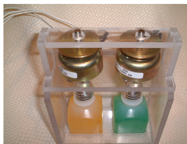
Figure 46: Dollars & Scents, showing the twin solenoids. The colors in the bottles are for photographic reasons alone.
