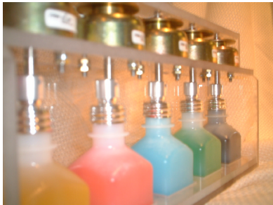
Figure 48: A five-channel aromatron, built for Scent Reminder. It was set up to output scents of baby powder, mint, rose, lemon and apple on demand. Colors are for photographic purposes alone.
