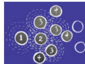
Illustration of the spread of a message within the Nami network.
