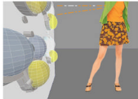
Diagram of the Furby™ pixel showing the infrared emitter, receiver and the speaker (hidden from view behind the front panel of the display).
