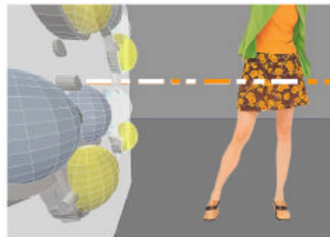
Each pixel uses an infrared detection circuit to probe for an observer in front on the display.
