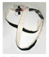
Figure 58: Breath sensor band The band is worn about the chest. A stretch sensor inside the band records the expansion and contraction of the chest cavity.
