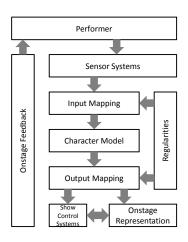
Figure 55: Disembodied Performance System overview diagram
