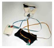
Figure 57: Arm gesture sensor assembly
