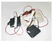
Figure 59: Shoe sensor assembly Two pressure sensors are attached to the sole of each shoe with elastic straps.
