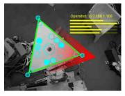
Figure 49: Operabot control view On an overhead image of the stage, the Core system overlays the status information and position icon for each Operabot. This view allows operators to monitor the robots and correct position and orientation discrepancies.
