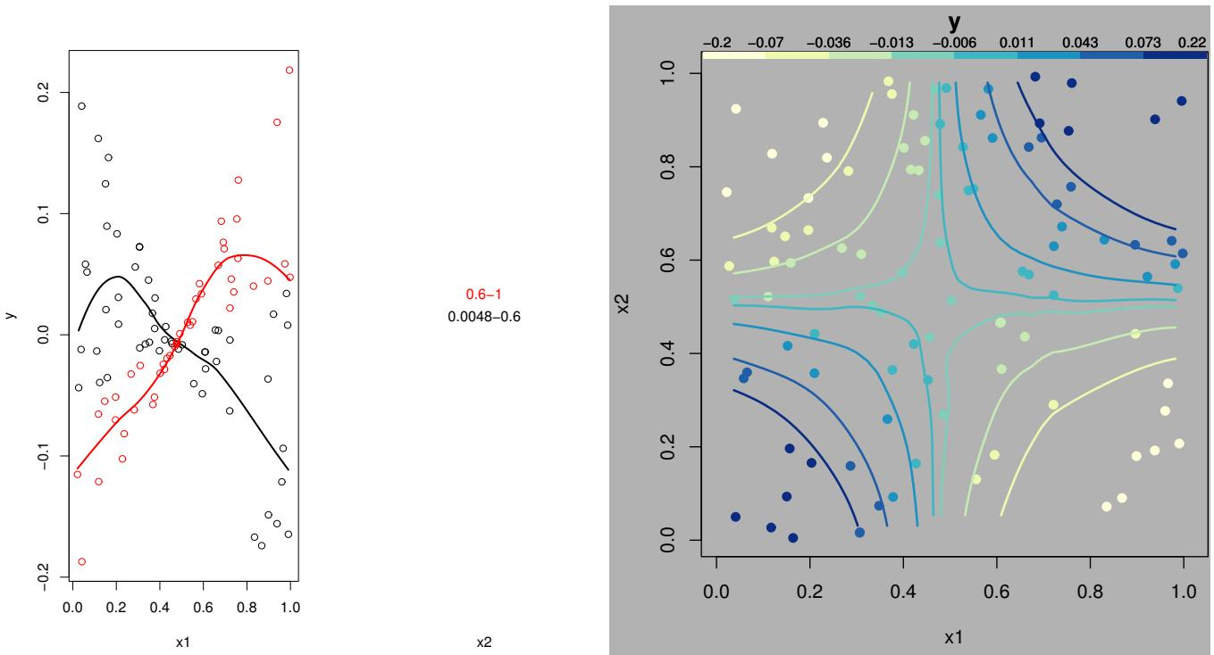
This data has formula  $y = x_1 + x_2 + x_1x_2$ . This is known as a **bilinear** interaction, because it is linear in each variable (notice how the slices have linear trends). It is easy to recognize this type of interaction from a contour plot. Using the definition in handout 5, it is a positive interaction, because knowing one variable makes the other more important.
